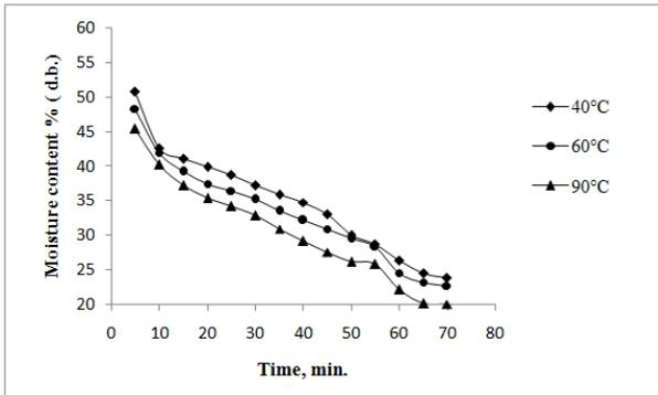
Fig. 3: Drying curve in FBD
