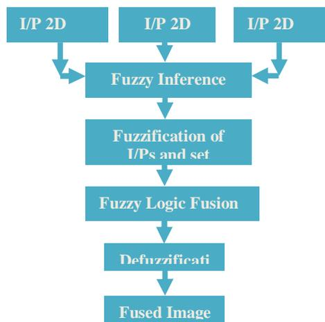
Figure 2. Block Diagram of Fuzzy Based Image Fusion
