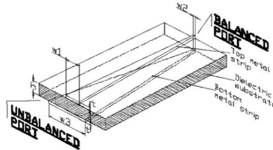
Fig.1. Linearly tapered microstrip balun.
