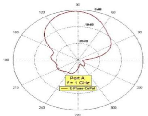
Fig.2 Measured E-plane radiation pattern of port A
