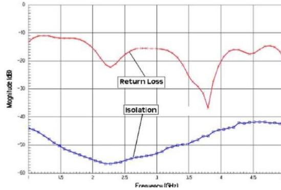
Figure. 5. Return loss and isolation of two ports of balun card, simulated with HFSS
