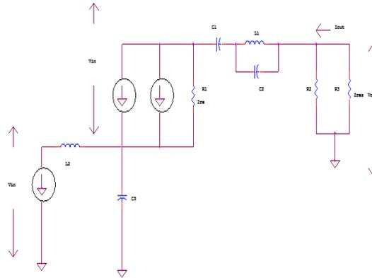
**Fig.3. Signal equivalent circuit**
