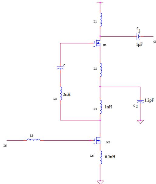
**Figure.4. Recycle mode Structure of Gain Optimization**
