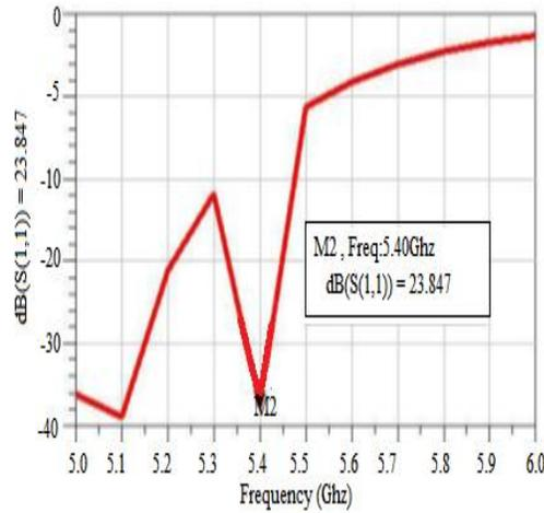
Figure.7. Input Side Reflection coefficient analysis
