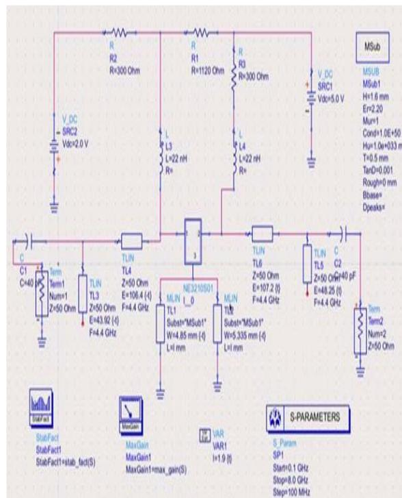
**Figure.3. Proposed Low Noise Amplifier (LNA)**
