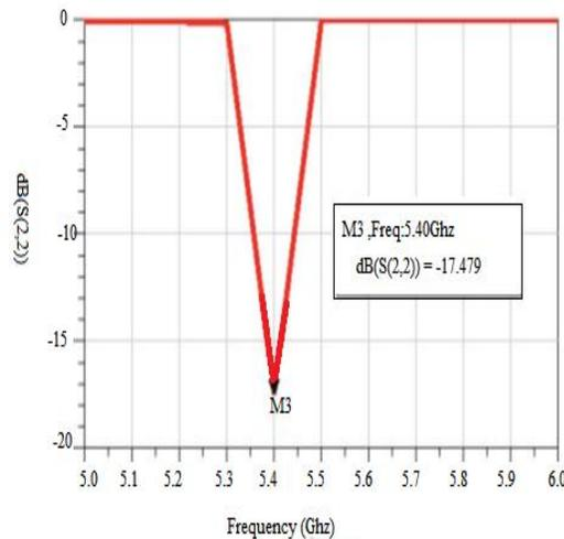
Figure.8. Output Side Reflection coefficient analysis
