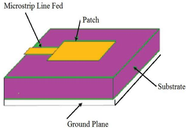
**Figure.1. Basic Structure of Micro Strip Antenna**
