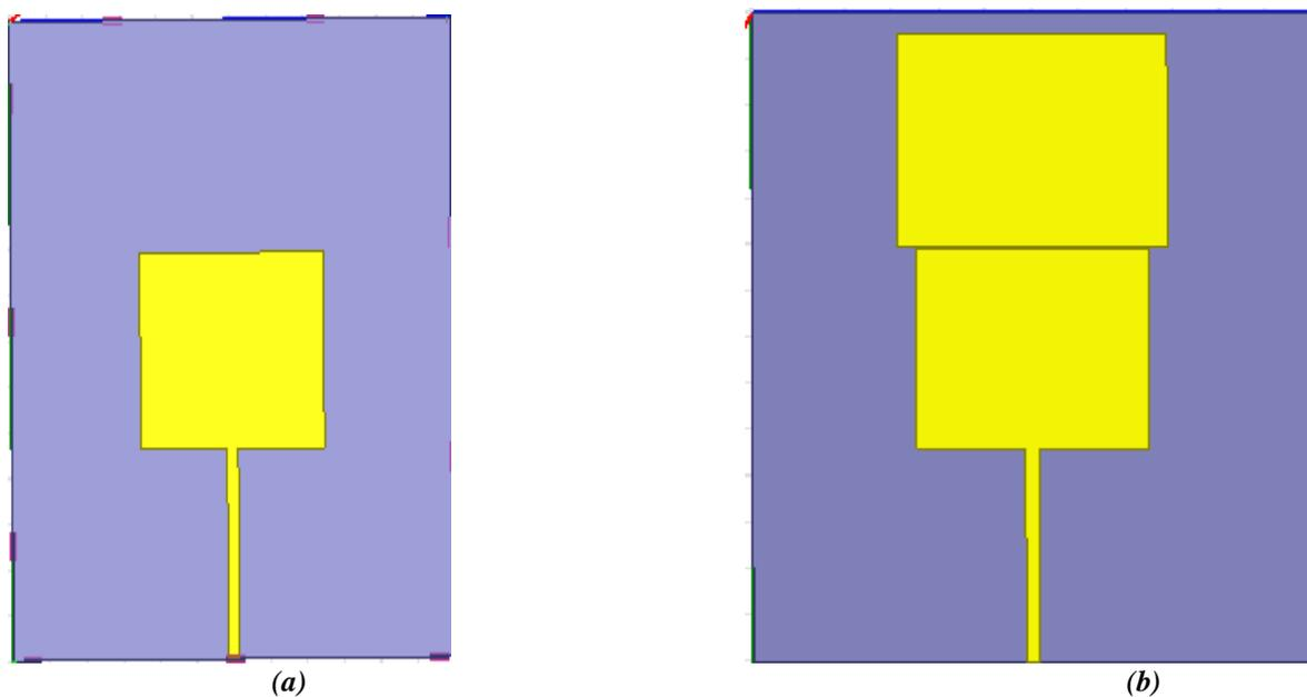
*Fig 1: Design evolution of (a) An Antenna without parasitic element, (b) An antenna with parasitic element*
