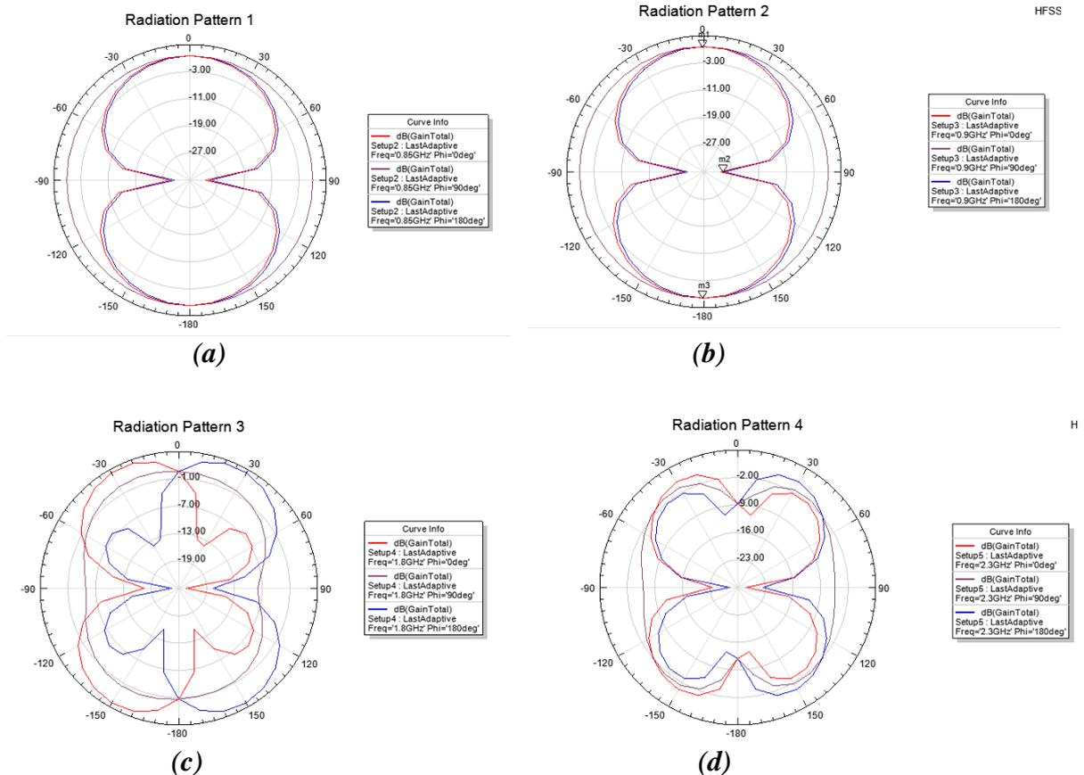
Fig 3: Radiation of proposed antenna (a)850MHz (b)900MHz (c)1800MHz (d)2300MHz
