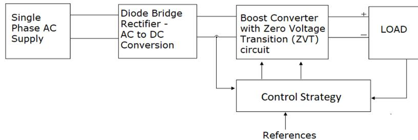
*Figure 1. Block diagram of proposed topology*
