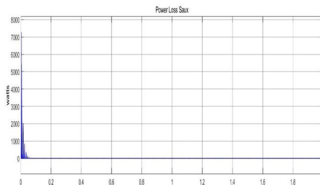
**Figure 12. Switching Losses at  $S_{aux}$**
