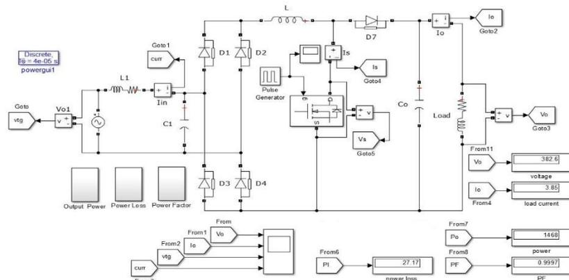
Figure 4. Boost converter simulation
