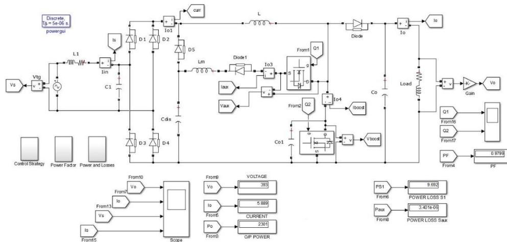
Figure 7. Closed loop simulation with ZVT circuit
