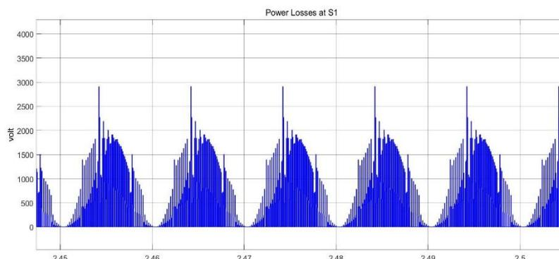
Figure 6. Power loss across switch S1
