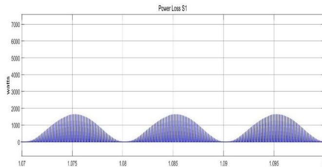
**Figure 11. Switching Losses at switch S1**
