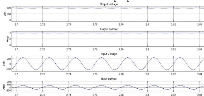
Figure 5. Waveforms of boost converter
