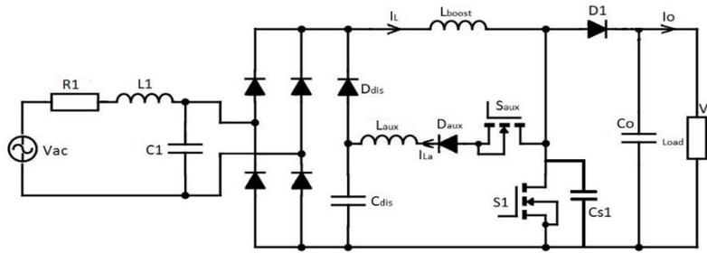
Figure 2. Circuit diagram of proposed topology
