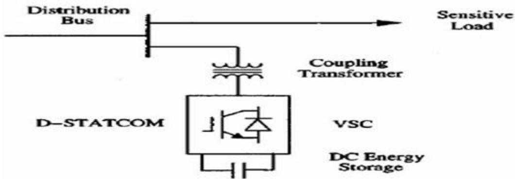
Fig 3 Distributions STATCOM (DSTATCOM)
