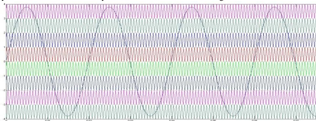
Fig.7 Reference and carrier waveform for nine level inverter
