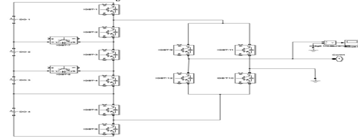
Fig.6. Multi-level Inverter Model
