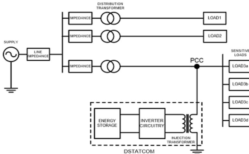
Fig.5: Typical Location of DSTATCOM in Distribution System
