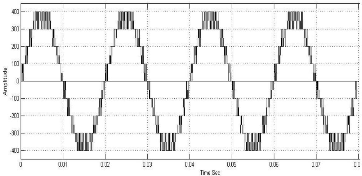
Fig.10. 9-level inverter output Voltage
