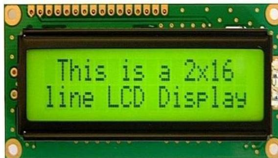
Fig.6. LCD Display
