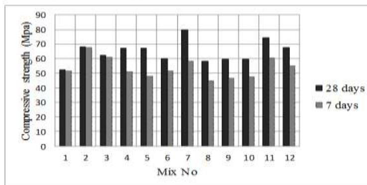
**Figure 5: Compressive strength of different mixes at 7- and 28-day ages.**
