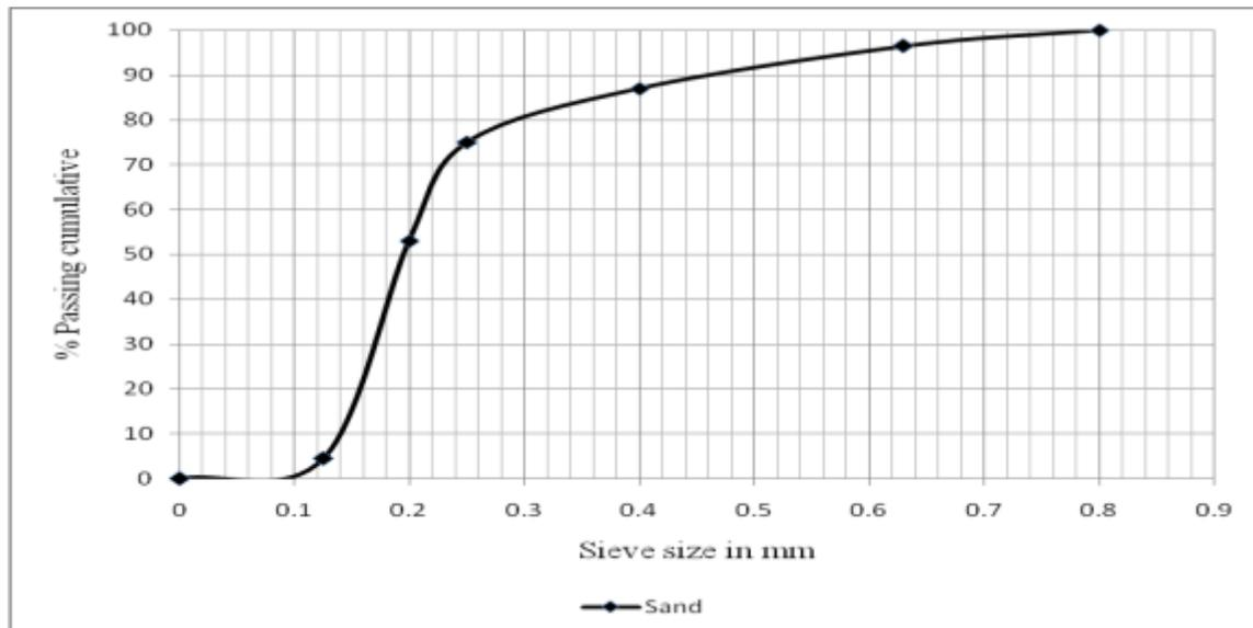
**Figure. 4: Sieve analysis of sand.**
