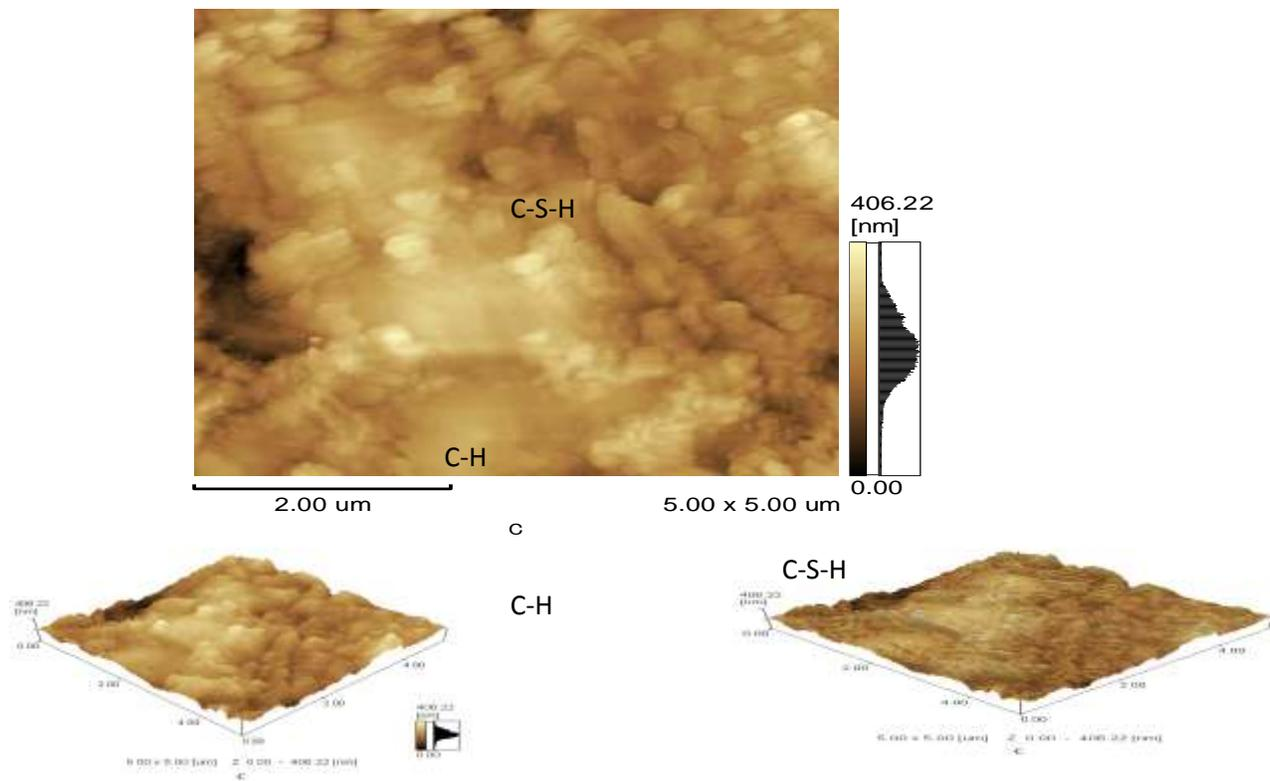
Figure. 8: AFM photographs of the control mix.
