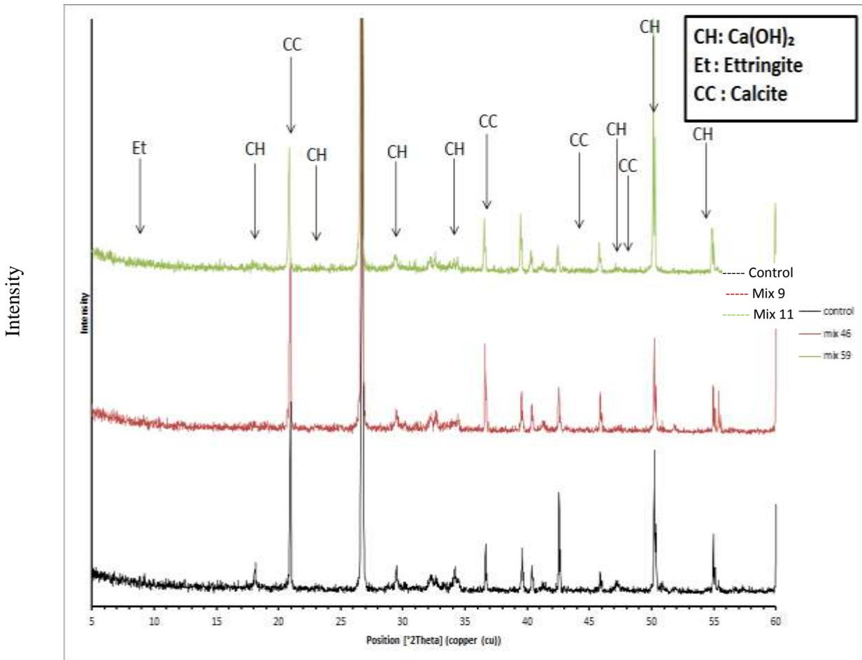
Figure. 13: XRD of control, # 9 and # 11 mixes.
