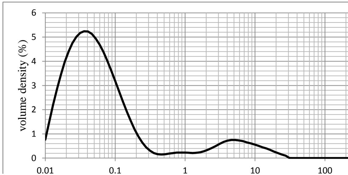
**Figure. (3): Particle size distribution of NS.**
