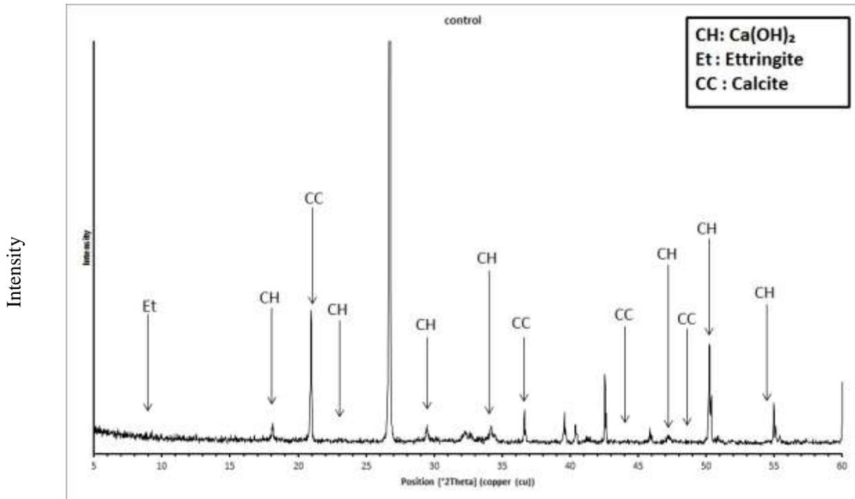
**Figure. 10: XRD of control mix.**
