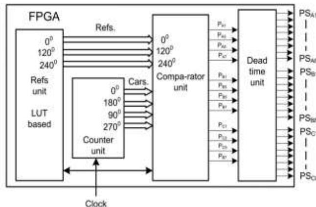
Figure 4 switching controller architecture
