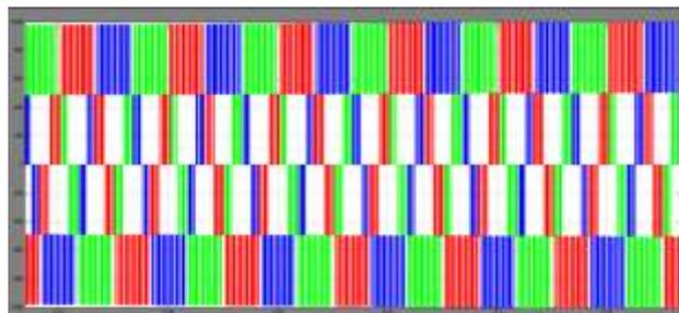
**Figure. 7. Simulated three phase line voltages of 1-kV multilevel cascaded converter**
