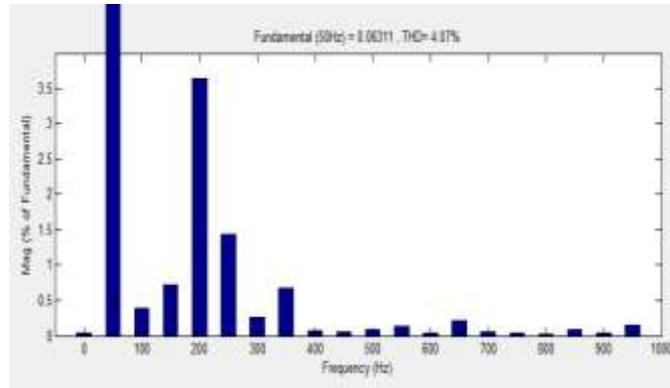
**Figure. 9. Frequency spectrum of line voltages**
