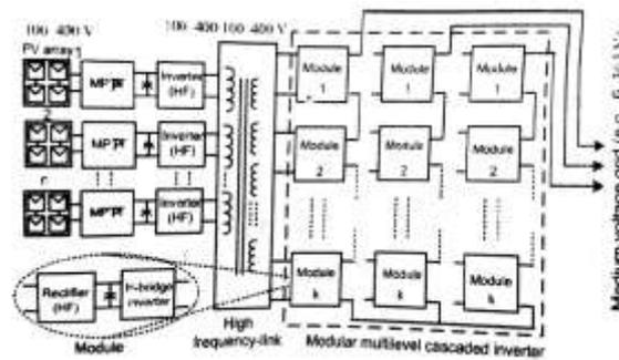
**Figure 1 Basic block diagram of proposed PV inverter system for direct medium voltage grid integration**
