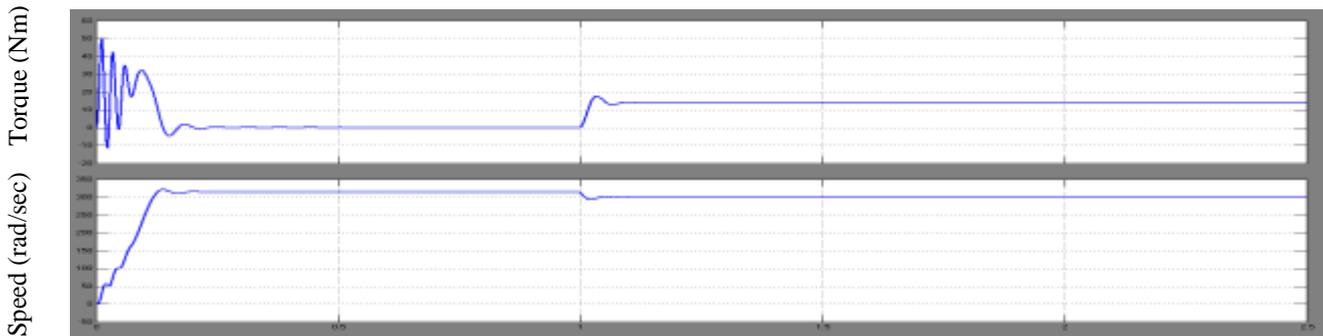
Figure 14: Torque and speed during under voltage condition at full load ( $T = 14Nm$ ) Time (sec)
