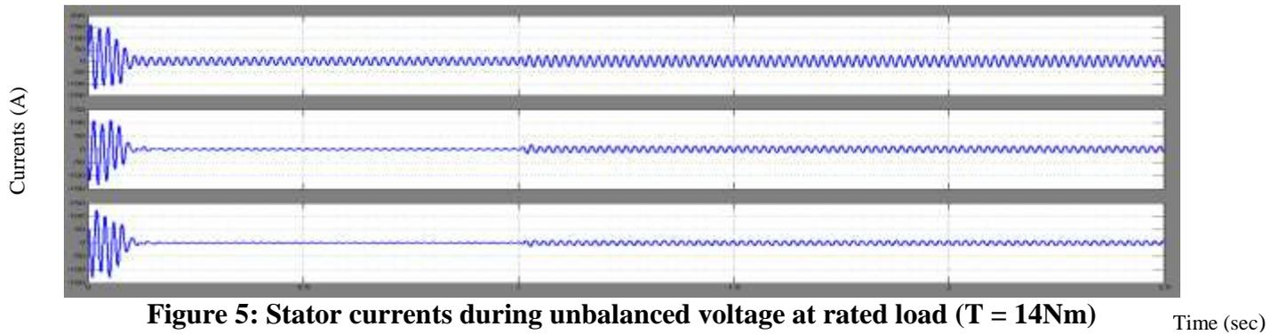
Figure 5 depicts the stator currents responses with respect to time during unbalanced voltage supply at rated load. Uneven distribution of stator phase currents is seen to be visibly high on application of rated load at one second with phase A having 25A, phase B having 13A and phase C having 9A. These excessive and unbalanced phase currents increase stator losses, reduce the motor efficiency and increase temperature rise, which could damage the windings of the motor.
