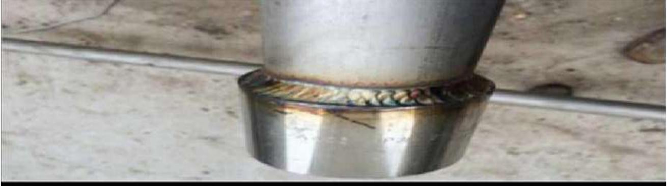
**Figure. 3 THE FIGURE SHOWS THAT TIG WELDED COMPONENT (SS316, SS102)**
