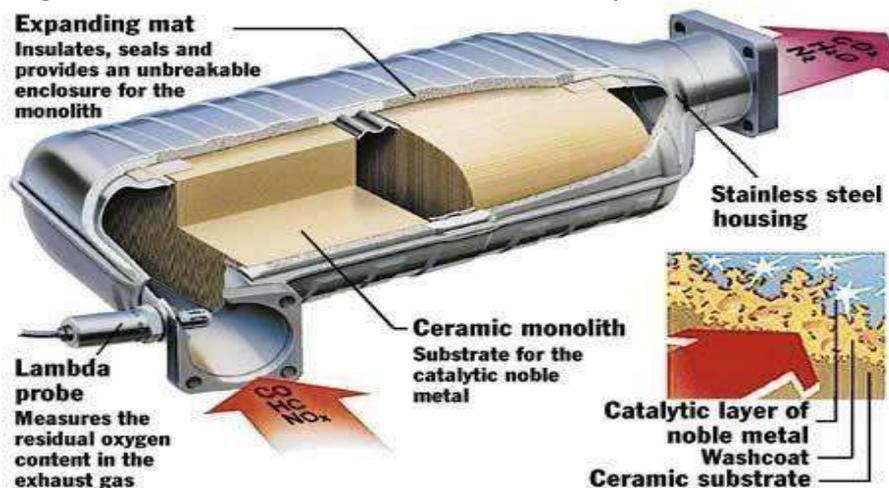
The carbon monoxide gas and hydrocarbons emitted from the engine will travel along the exhaust system until they reach their catalytic converter. There it comes into contact with the described catalyst. This forces a reaction between the carbon monoxide and hydrocarbons with the oxygen inside the converter creating products of carbon dioxide and water vapor. The reaction which occurs inside the converter is as follows:
