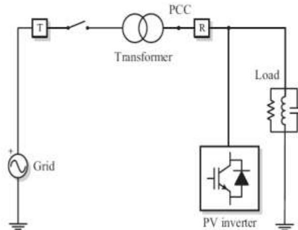
**Figure 4: After islanding (Load is fed by inverter in off grid mode)**
