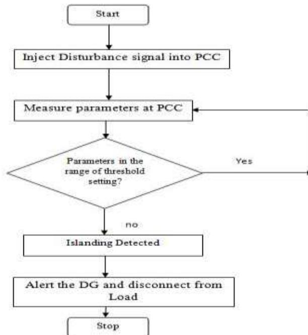
**Figure 2: Flowchart of Active Islanding Detection Methods.**
