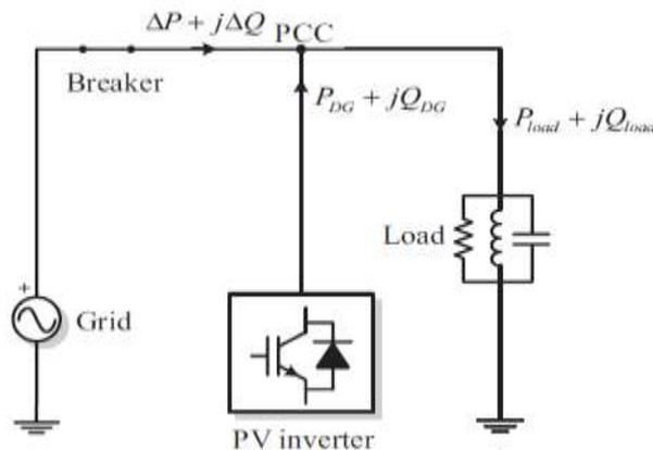
**Figure 3: Before Islanding (Load is fed by inverter in on-grid mode)**
