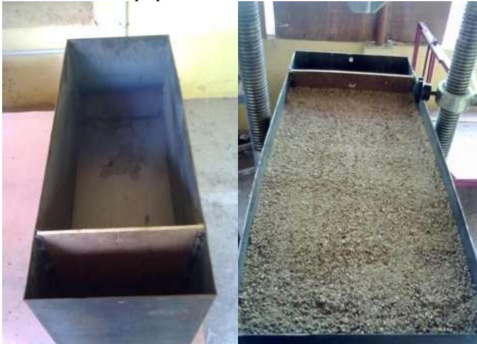
**Figure. 1 - Model tank with vertical facing    Figure. 2 -Tank filled with sand**
