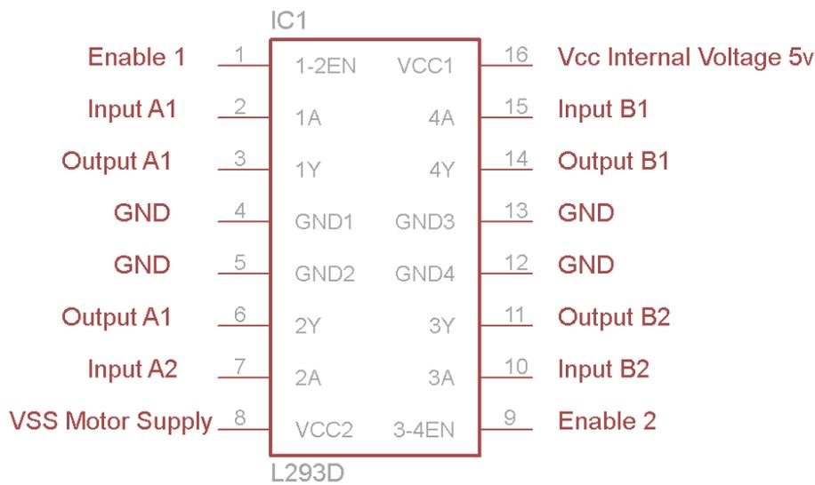
**Figure 8 L293D Pin Diagram**
