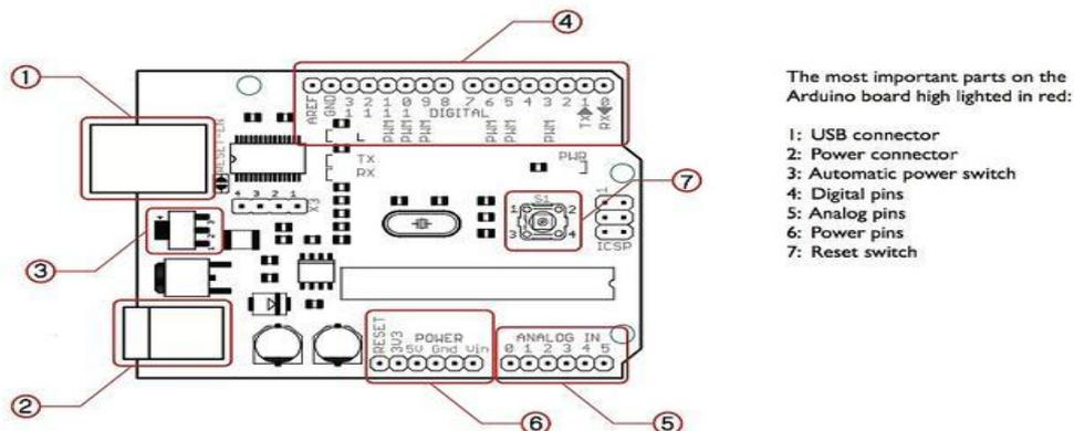
**Figure 4 Arduino Pin Diagram**
