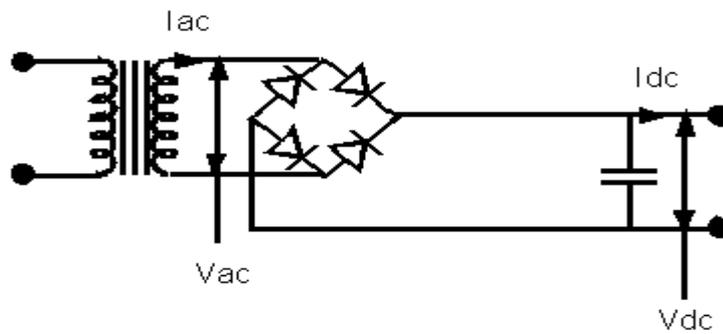
**Figure 2 Bridge Rectifier**
