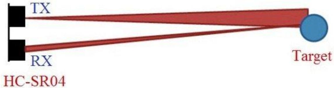
*Figure 6 HC-SR04 Ultrasonic Sensor operation*
