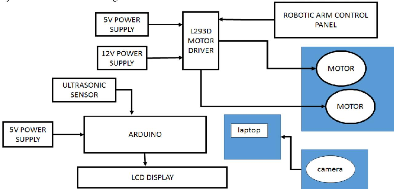
*Fig 1 Block diagram for the bore well rescue system*
