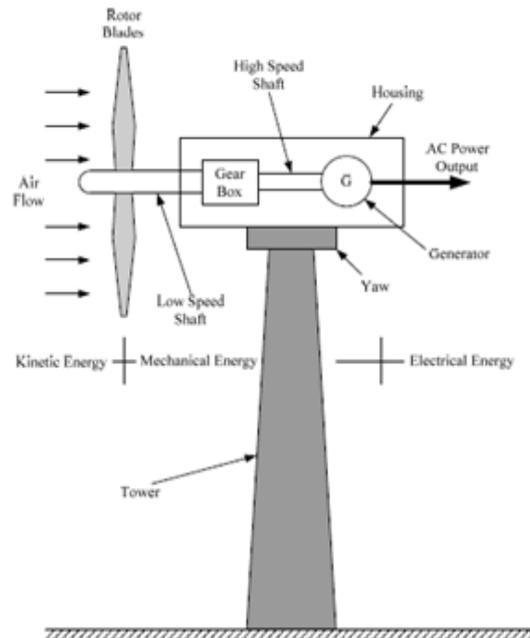
**Figure 1. Typical wind energy conversion system**
