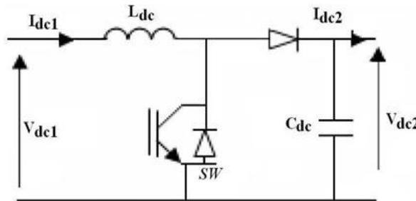
Figure 8. Boost (DC-DC) converter
