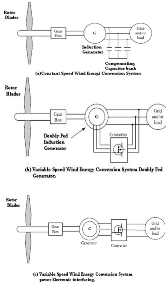
Figure 2. constant and variable speed wind energy conversion system
