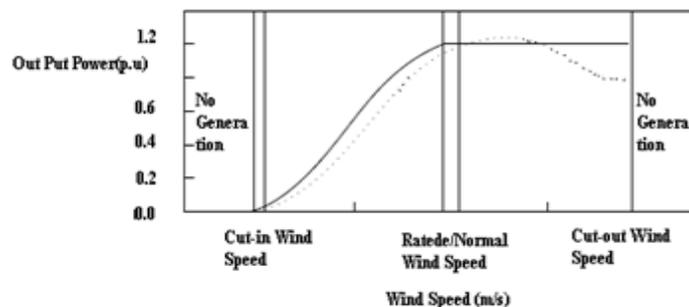
Figure 3. Typical curves for a constant speed stall controlled (dotted) and variable speed pitch controlled wind turbine
