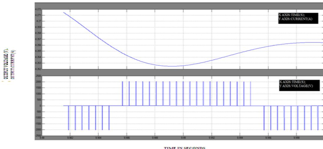
**Figure 12 .Inverter voltage and current waveform**
