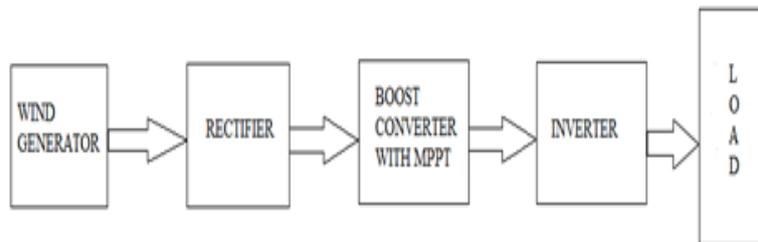
**Figure 6. Block diagram of the maximum power point tracking for wind energy conversion system**
