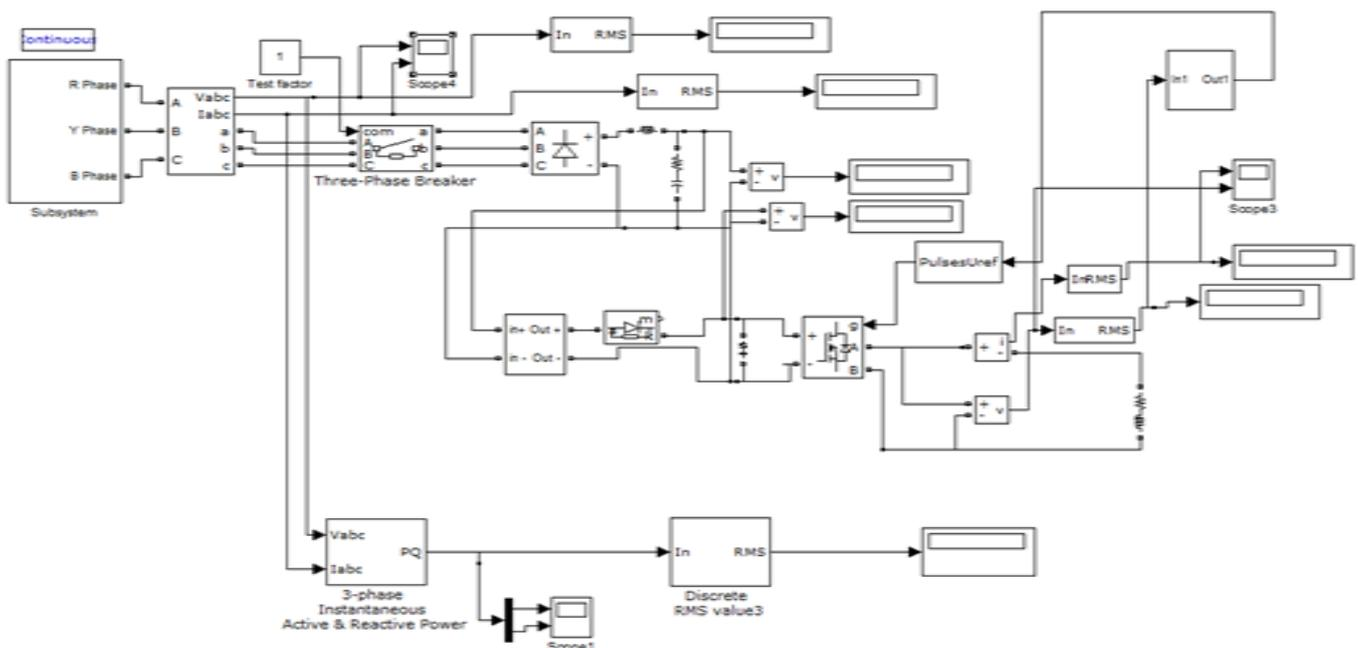
Figure 9. Simulation model of MPPT for Wind Energy Conversion System
