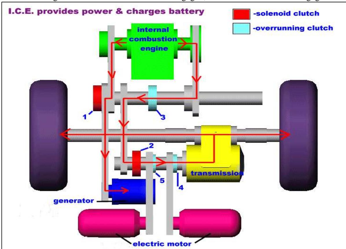
*Fig 4.5 I.C.E provides power and charges battery*
