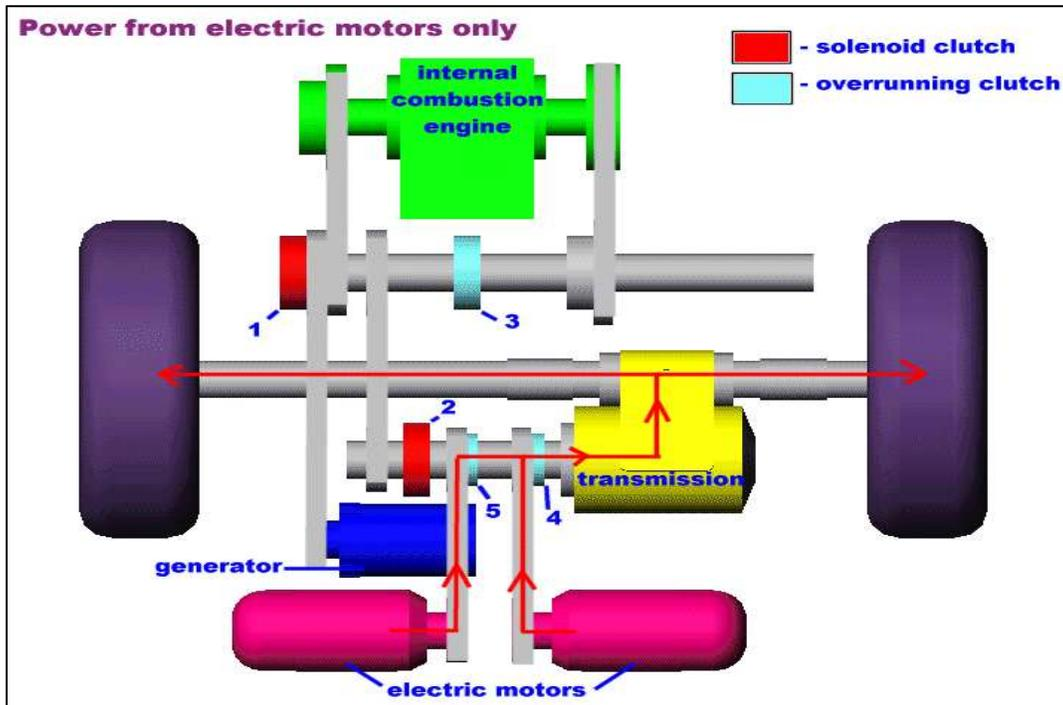
Fig 4.2 Power from Electric motors only
