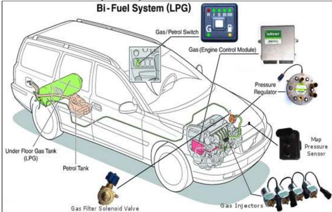
**Fig 1.2 Components of LPG hybrid system**
