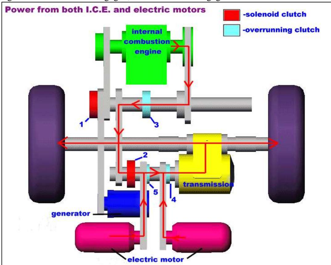
Fig 4.3 Power from both Motors and I.C.E
