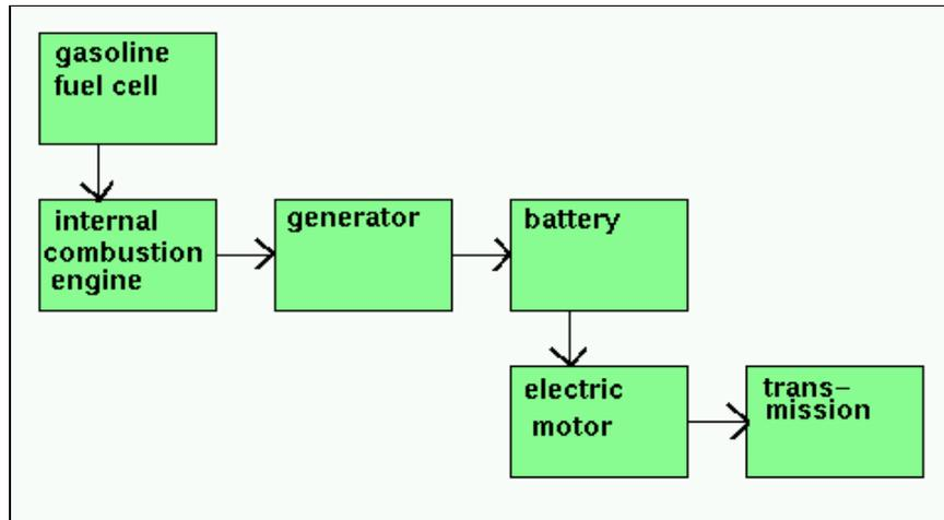
Fig 4.1 Configuration of series HEV
