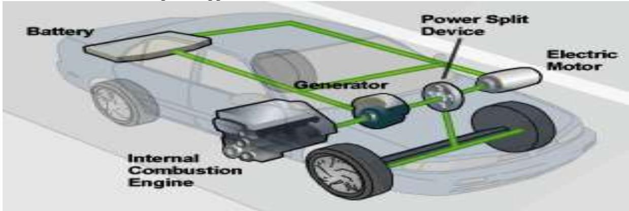
*Fig 1.4 various parts of electrical hybrid system*
