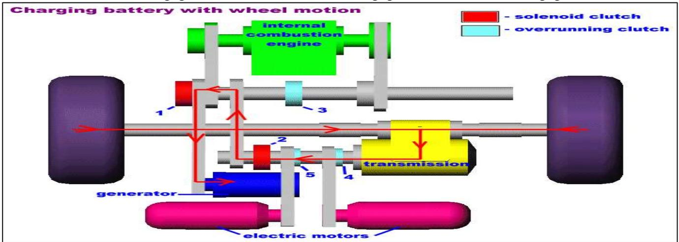
*Fig 4.4 Charging batteries with wheel motion*
