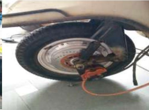
*Fig 9.2 Hub Motor with independent brake*
