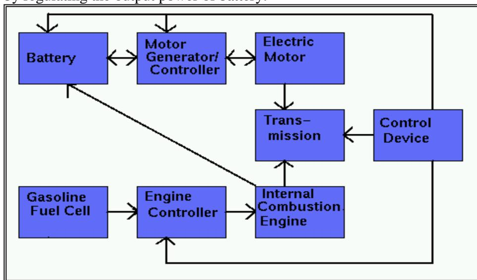
Fig 4.2 Configuration of parallel HEV
