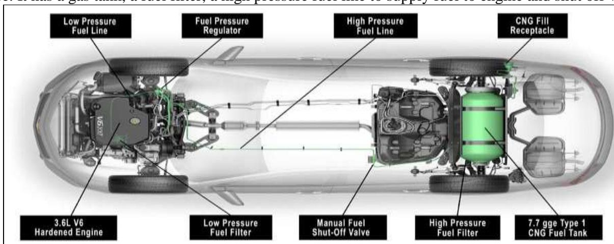
*Fig 1.1 Components of CNG hybrid system*
