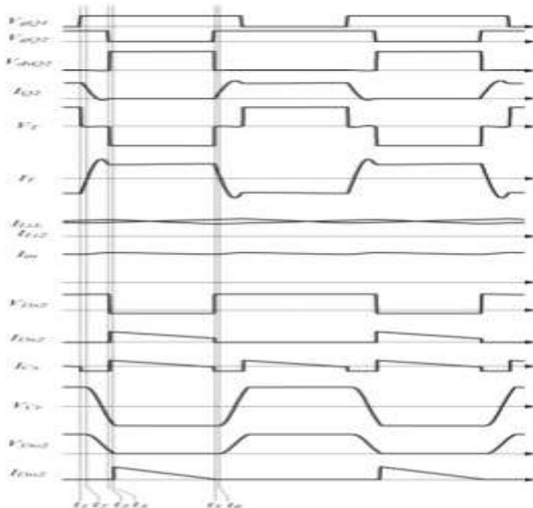
Figure 3. Key waveforms of TIBC during switching period
