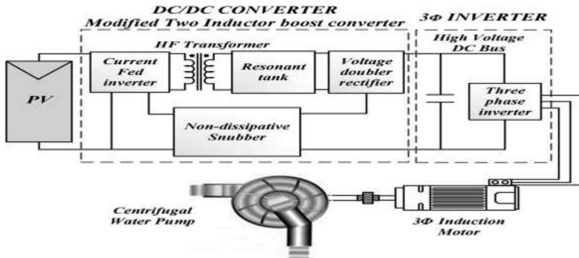
Figure 1. Simplified Block Diagram of the Proposed System
