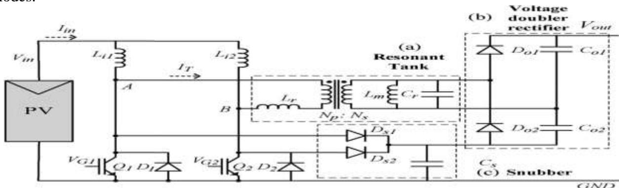
Figure 2. Modified TIBC topology: (a) resonant tank, (b) voltage doubler rectifier and (c) snubber.
