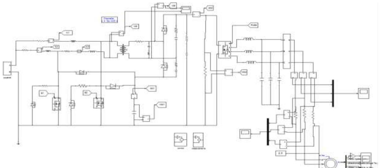
Figure 5. Circuit used for the Implementation of Photovoltaic Converter for Water Pumping System
