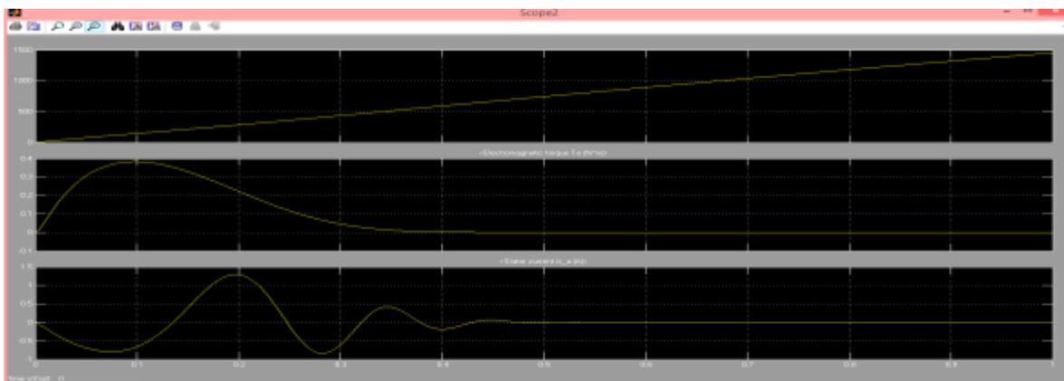
*Figure 10. Rotor speed, Electromagnetic torque, Stator current*
