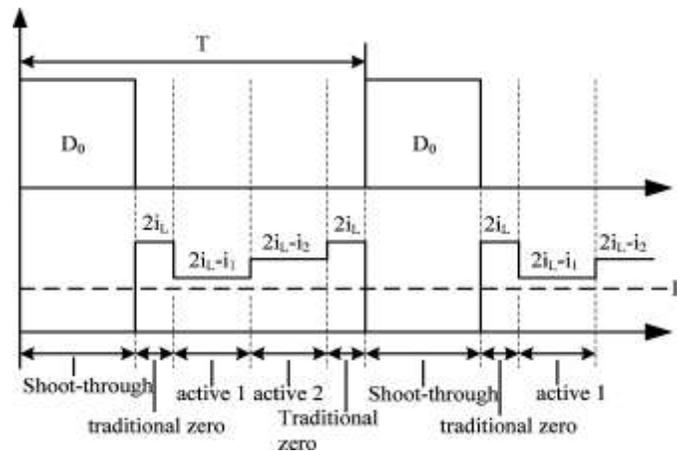
Fig. 6. Input current of the traditional Z-source inverter.
