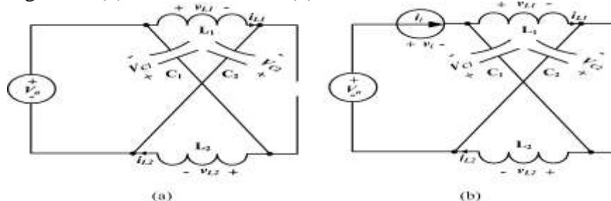
Fig. 4. Equivalent circuit of improved Z-source inverter. (a)Shoot-through state. (b) Non-shoot-through state.
