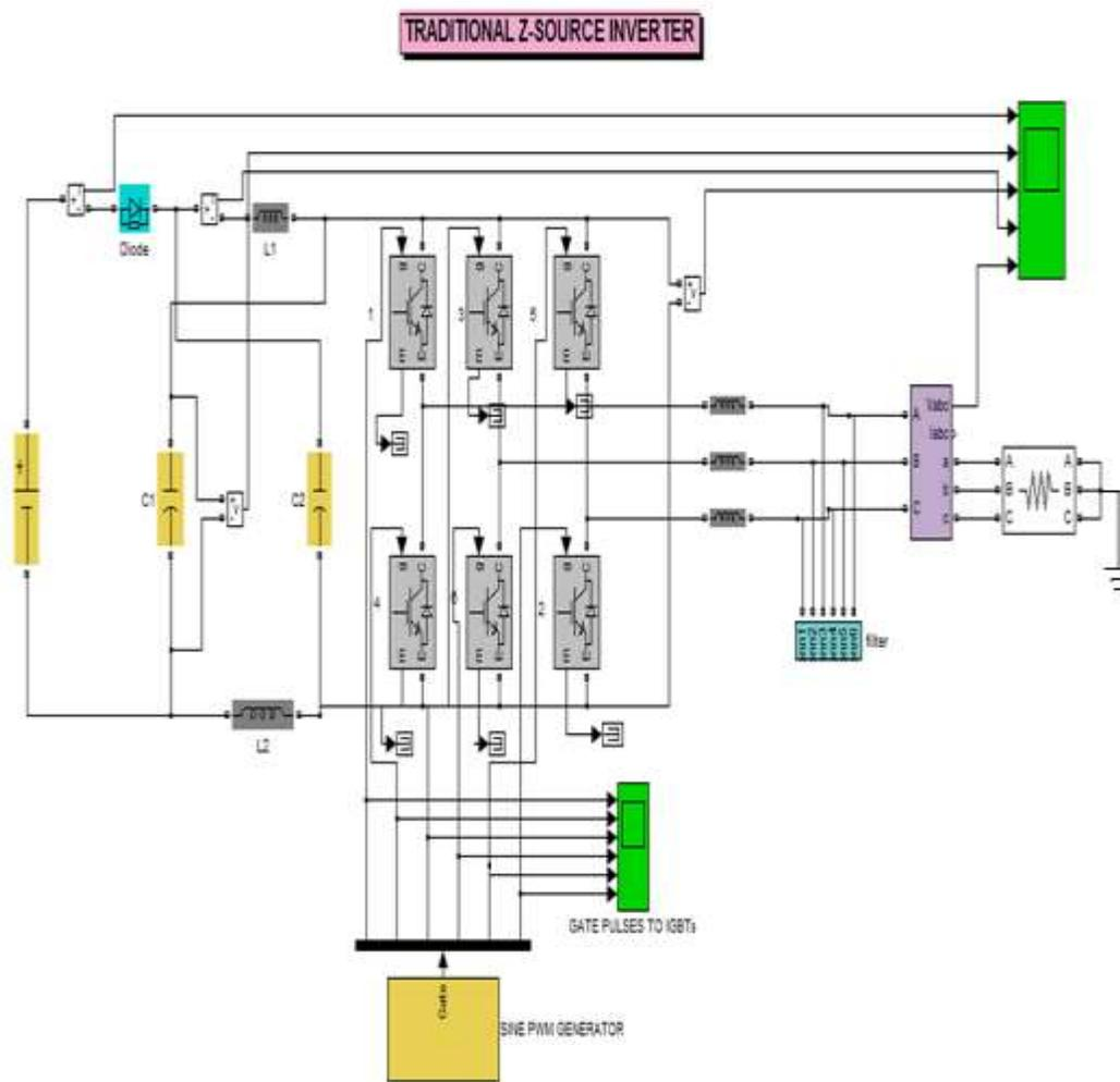
**Fig. 1.** Z-source inverter.
