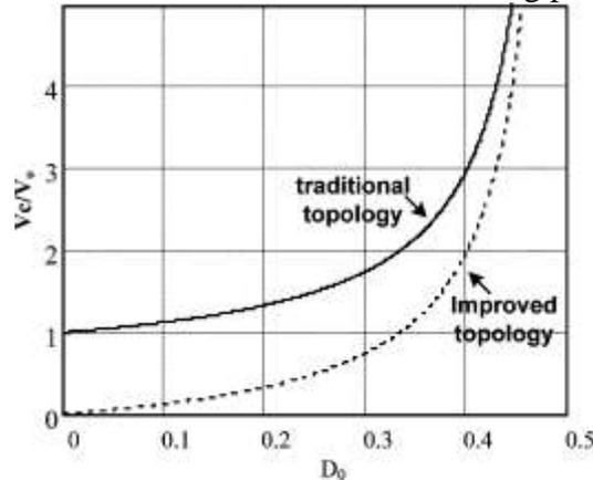
Fig. 5.  $V_C/V_0$  versus  $D_0$  of the two topologies.
