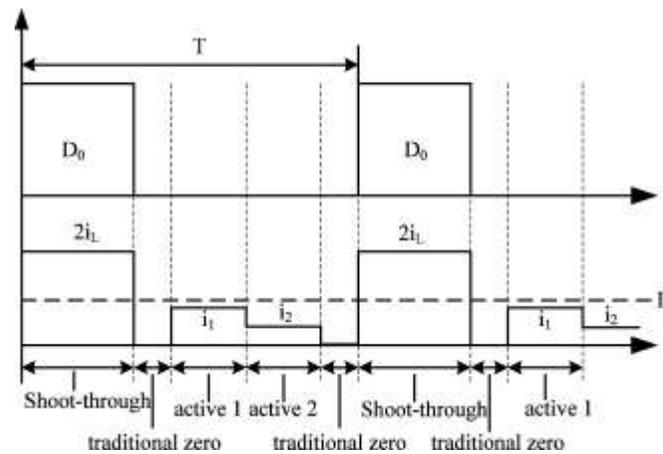
Fig. 7. Input current of the improved Z-source inverter.
