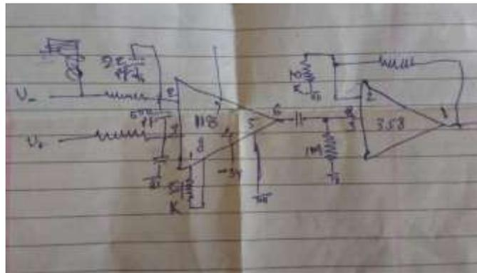
Figure 4. ECG sensor module
