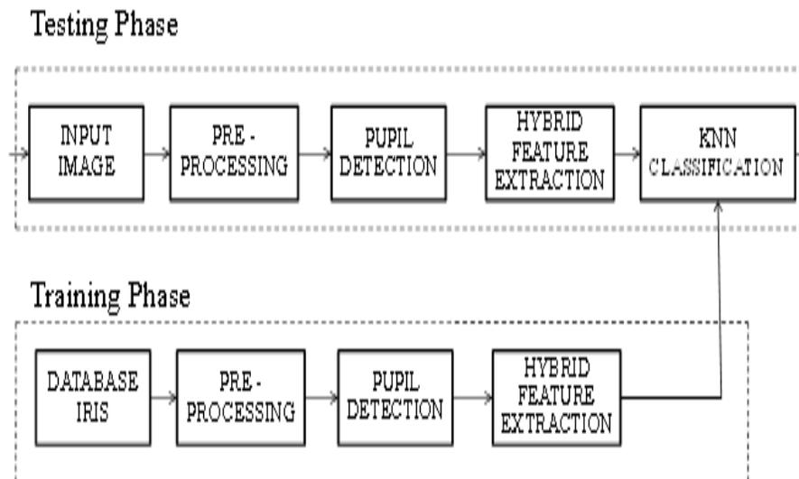
**Fig 1 : Block diagram of proposed system**
