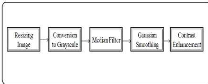
**Fig 3: Block diagram of Preprocessing stage**
