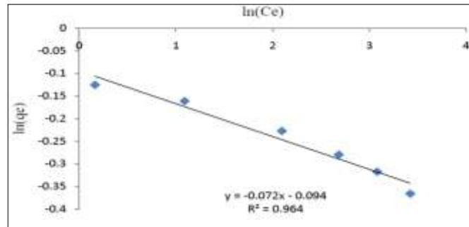
Figure 7: Freundlich adsorption isotherm for Zn adsorption
