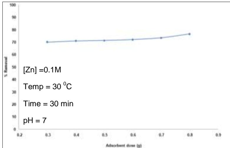
**Figure 3: Effect of adsorbent dose on adsorption of Zn**
