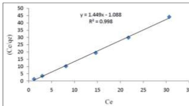
**Figure 6: Langmuir adsorption isotherm for Zn adsorption**
