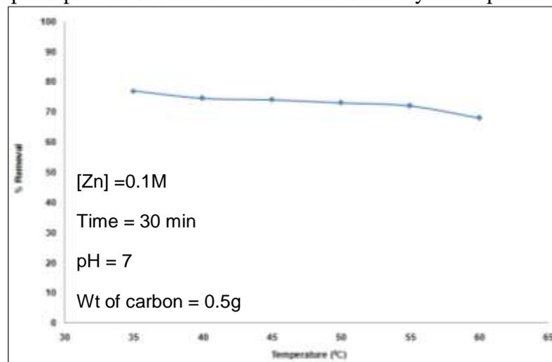
**Figure 4: Effect of temperature on adsorption of Zn**
