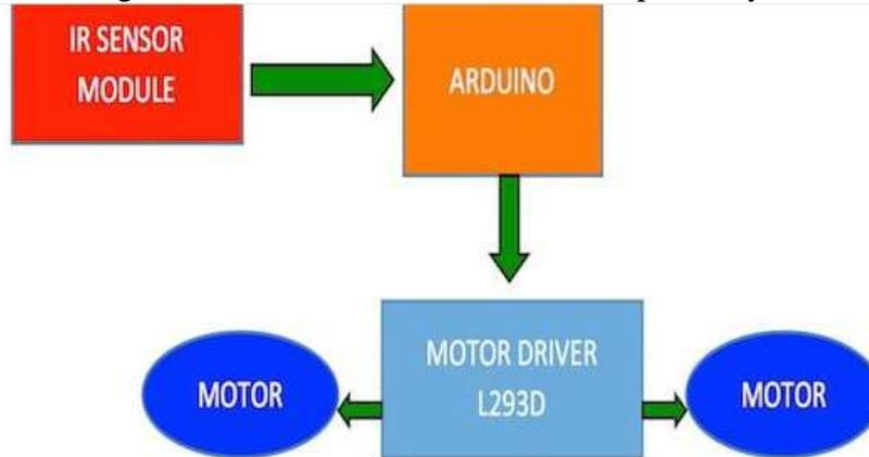
Figure 1:-Block diagram of the entire project
