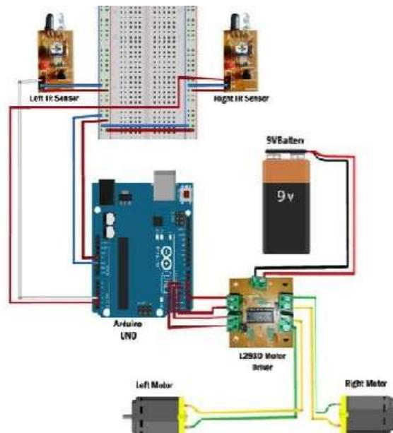
Figure:-2 Circuit diagram of the project
