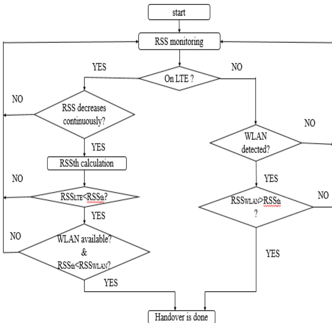
**Figure 2. RSS threshold Handover algorithm**
