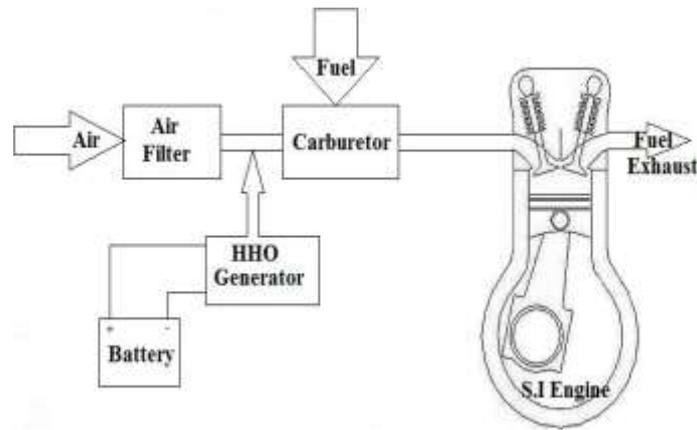
fig.(1) Working Principle
