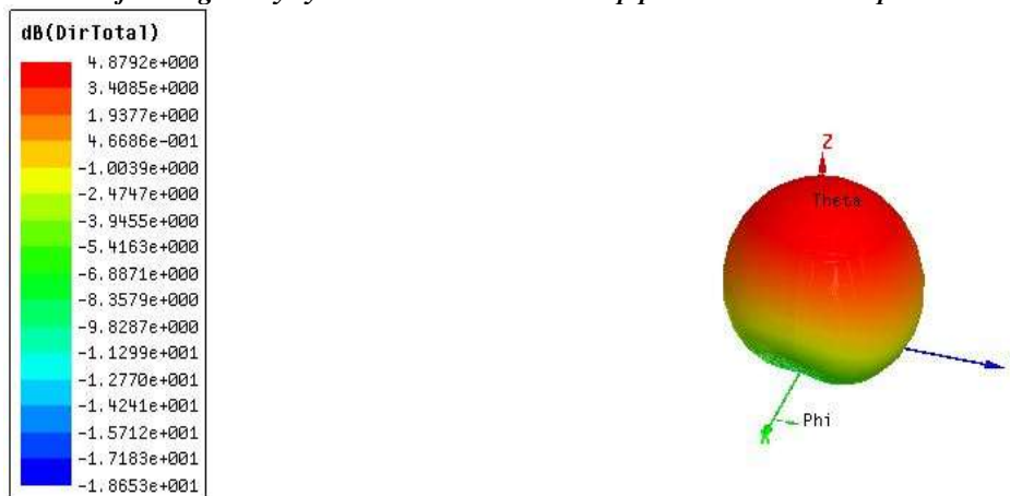
Figure 11.Directivity for diagonally symmetric slotted microstrip patch antenna with plus slots at 3.7Ghz
