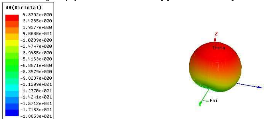
Figure 9.Directivity for diagonally symmetric slotted microstrip patch antenna with plus slots at 2.4Ghz
