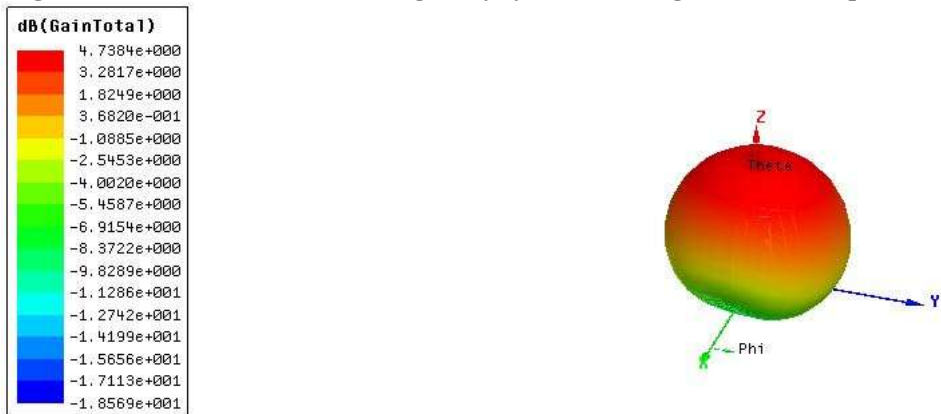
Figure 13. Gain for diagonally symmetric slotted microstrip patch antenna with ring slots at 1.17GHz
