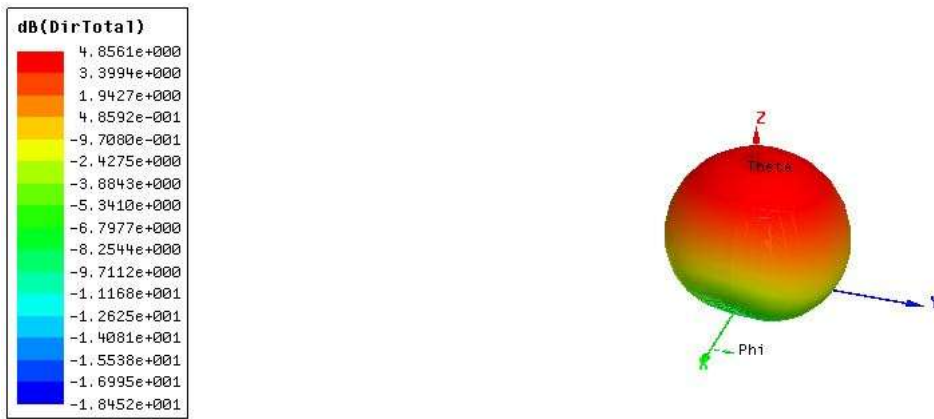
Figure 16 Directivity for diagonally symmetric slotted microstrip patch antenna with ring slots at 2.4Ghz
