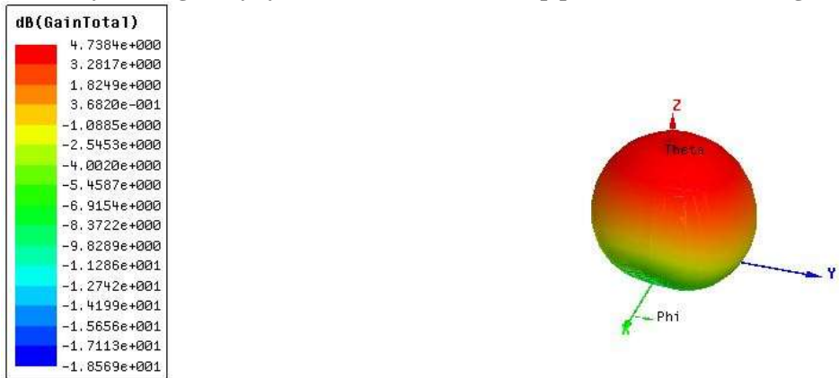
Figure 17.Gain for diagonally symmetric slotted microstrip patch antenna with ring slots at 3.7Ghz
