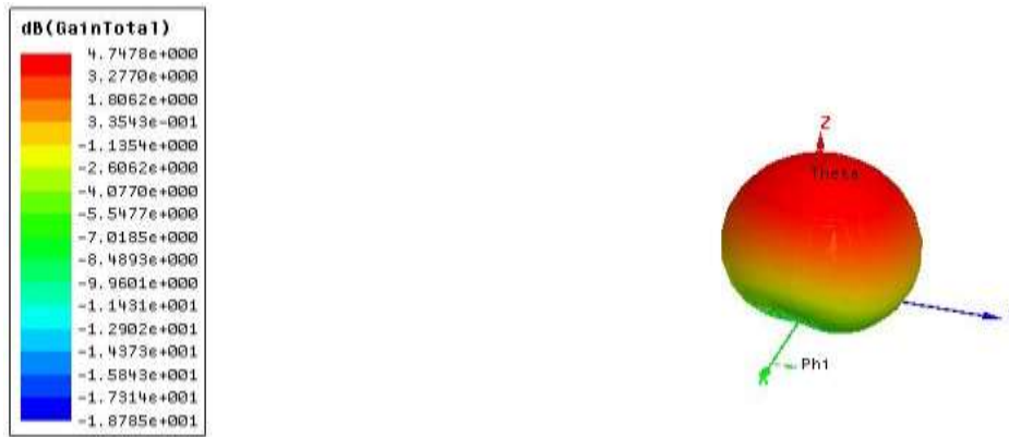
Figure 8.Gain for diagonally symmetric slotted microstrip patch antenna with plus slots at 2.4Ghz
