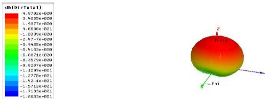
Figure 6. Directivity for diagonally symmetric slotted microstrip patch antenna with plus slots at 1.17GHz
