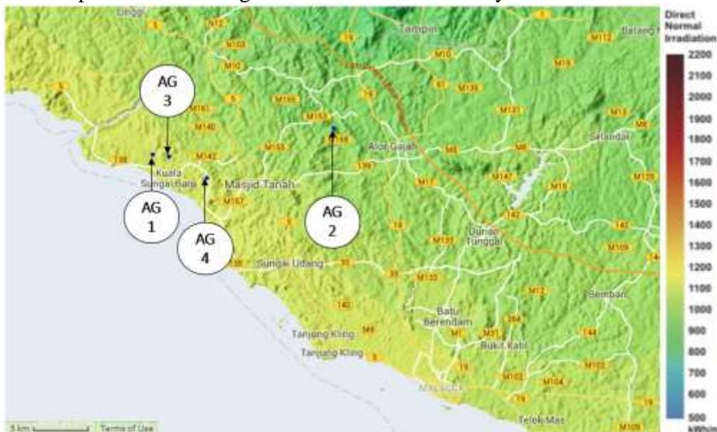
Figure 5. DNI data mapping for locations experimented in Alor Gajah by SolarGIS
