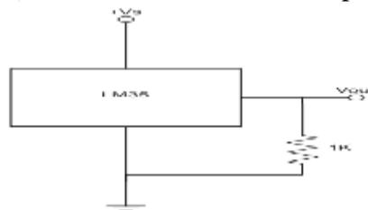
**Fig.3. Connection of LM35 temperature sensor**
