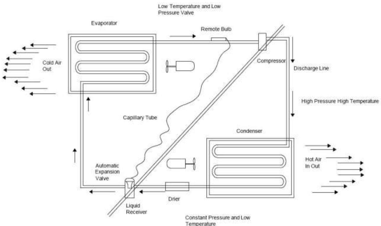
**Fig.1 Refrigeration and Air conditioning System**
