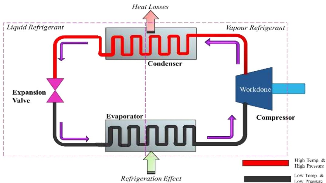
Fig. 1. Schematic diagram of simple VCR System
