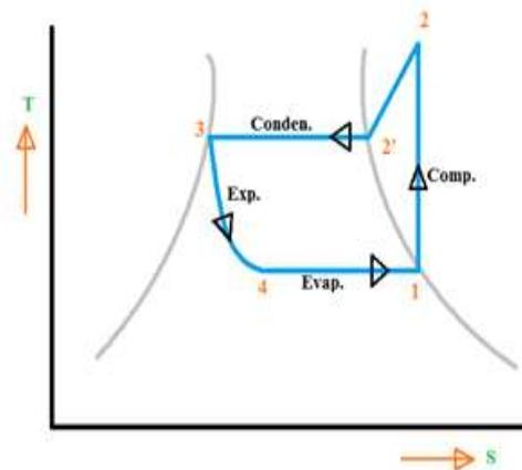
Fig. 3: T-S diagram of VCRC
