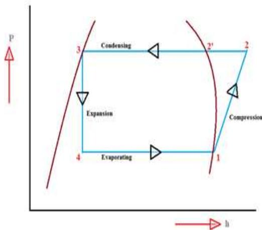
Fig. 2: P-h diagram of VCRC
