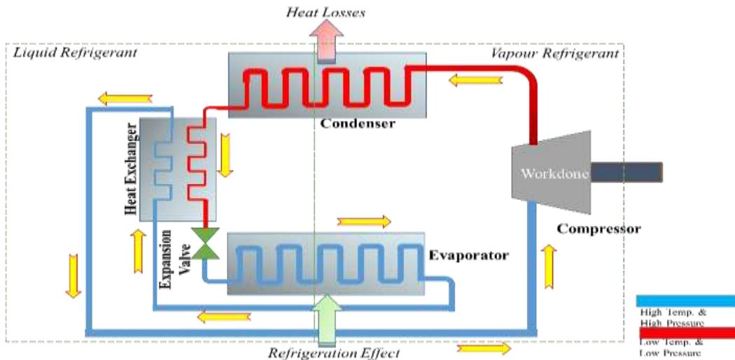
Fig. 4. Schematic diagram of simple VCR System with Heat Exchanger
