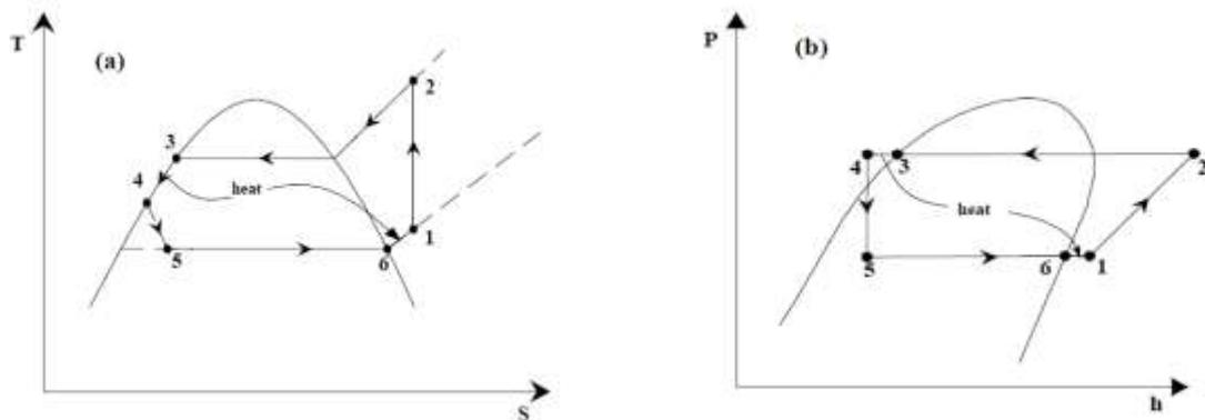
Fig. 5. Single stage Vapour Compression Refrigeration System cycle with LSHX (a) On T-s diagram (b) on P-h diagram
