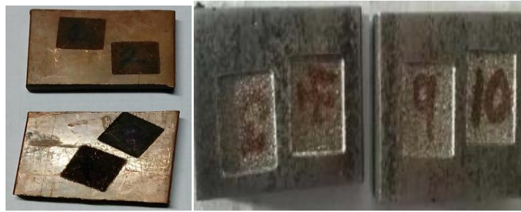
Figure 2. (a)Copper work pieces (b) High speed steel work pieces
