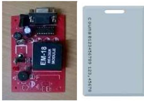
**Fig 4.1 EM-18 RFID Reader and Passive Card**
