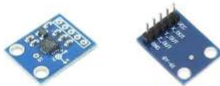
**Fig 4.2 ADXL335 Accelerometer**
