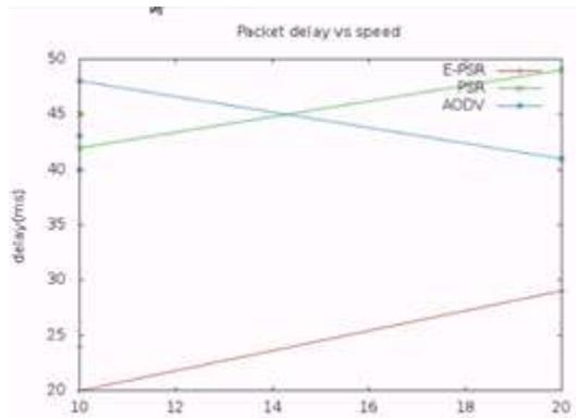
**Fig.6: Comparison graph for packet delay vs. speed**
