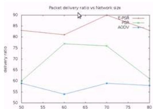
**Fig.8: Comparison graph for Packet delivery ratio vs. network size**
