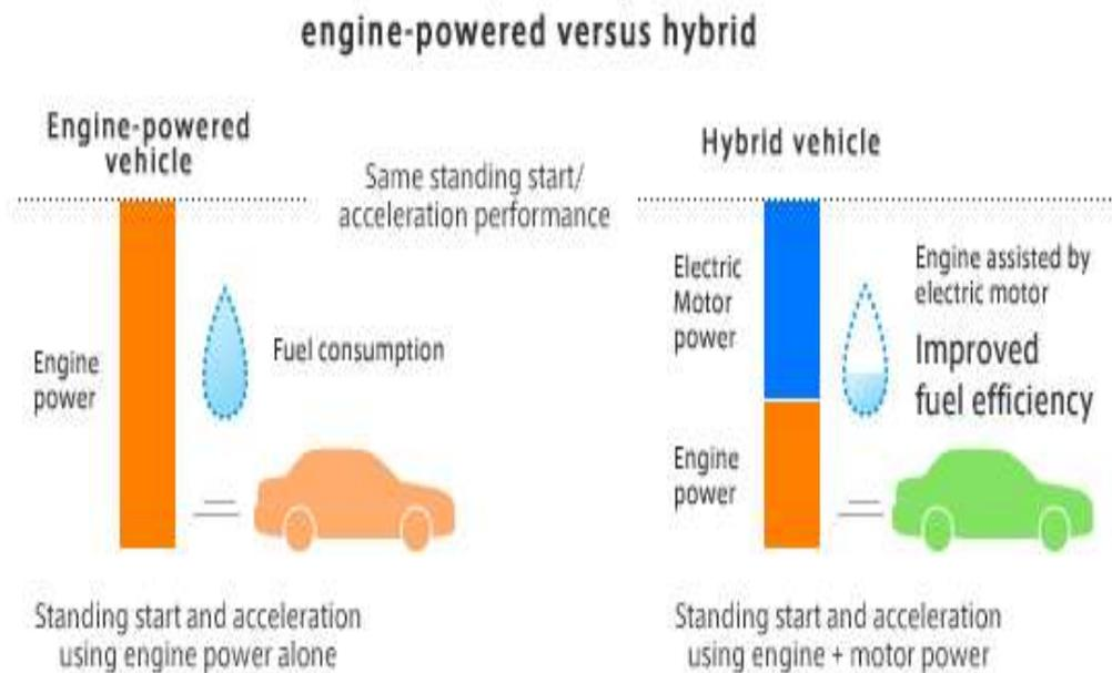
*Fig. 5 Comparison of conventional and hybrid vehicle*
