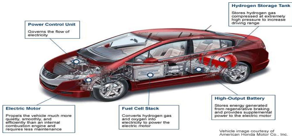
*Fig. 3 various parts of hydrogen fuel system*
