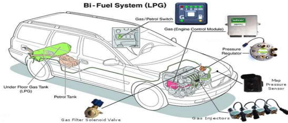
*Fig. 2 Components of LPG hybrid system*
