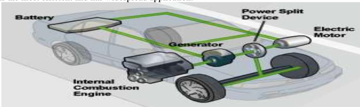
*Fig. 4 various parts of electrical hybrid system*
