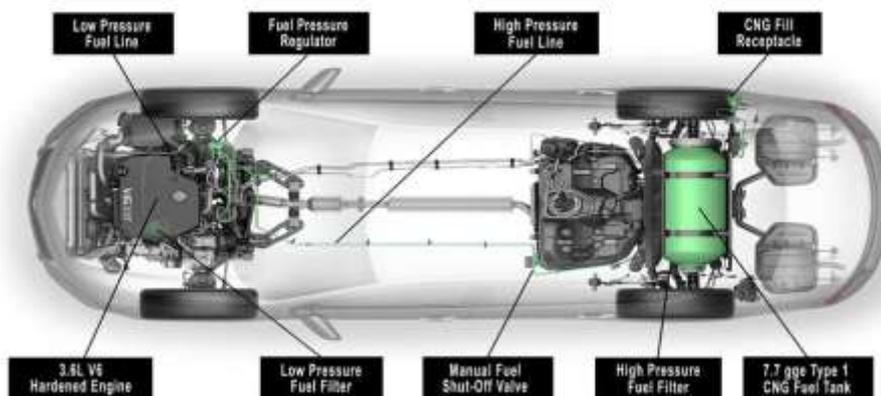
*Fig. 1 Components of CNG hybrid system*
