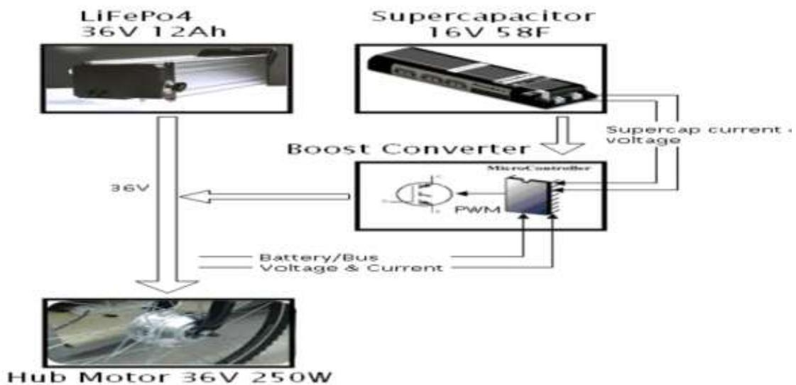
*Fig. 8 working of hybrid electric vehicle*
