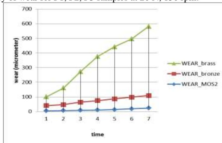
Figure 5. Comparative Study of Wear for 20 N, 150 Rpm
