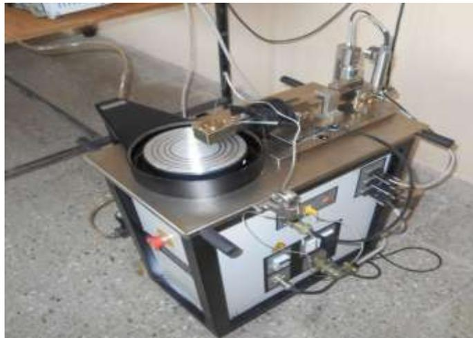
**Figure 3. Wear and friction measuring test rig TR-20**
