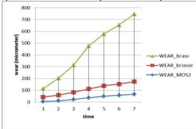
Figure 6. Comparative Study of Wear for 30 N, 200 Rpm
