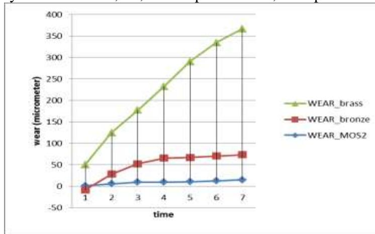
Figure 4 . Comparative Study of Wear for 10 N, 100 Rpm
