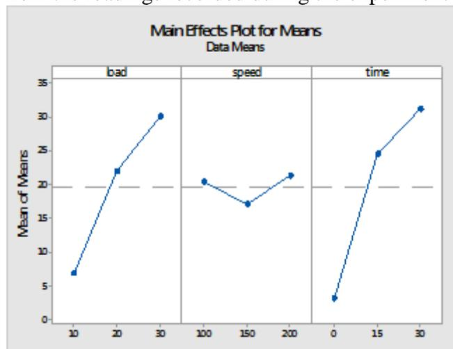
Figure 7. Main Effects Plot for Wear
