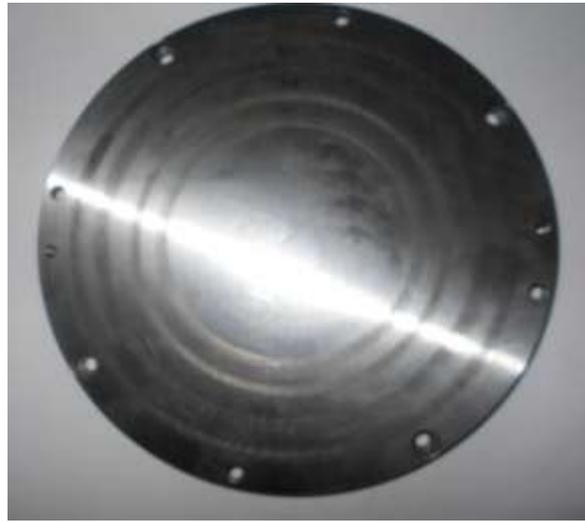
**Figure 2. EN 8 Disc With Size  $\varnothing$  165 $\times$ 8 mm**
