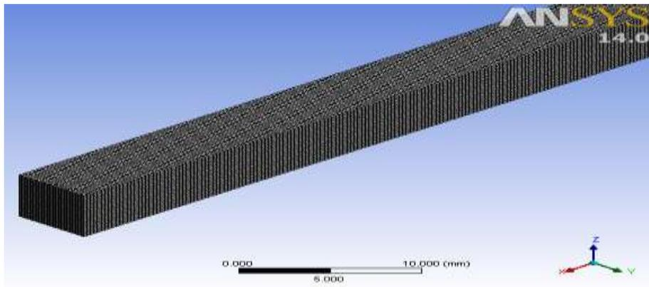
Fig 3: Unstructured mesh for 3D analysis of heat transfer without rectangular ribs
