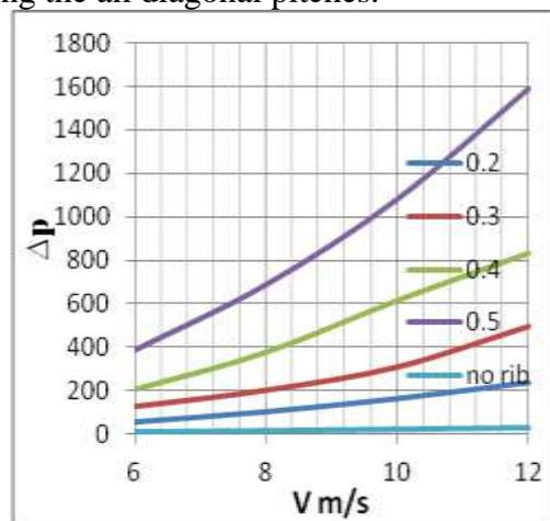
Fig 5.10(b):  $\Delta p$  v/s V plot for all pitches
