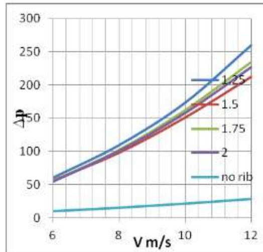
Fig 5.11(b):  $\Delta p$  v/s V plots for rib length 0.2 & 0.3.
