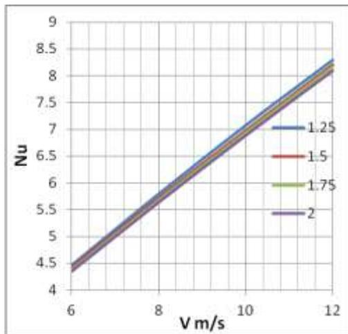
Fig 5.6(a): Nu v/s V plot for rib length
