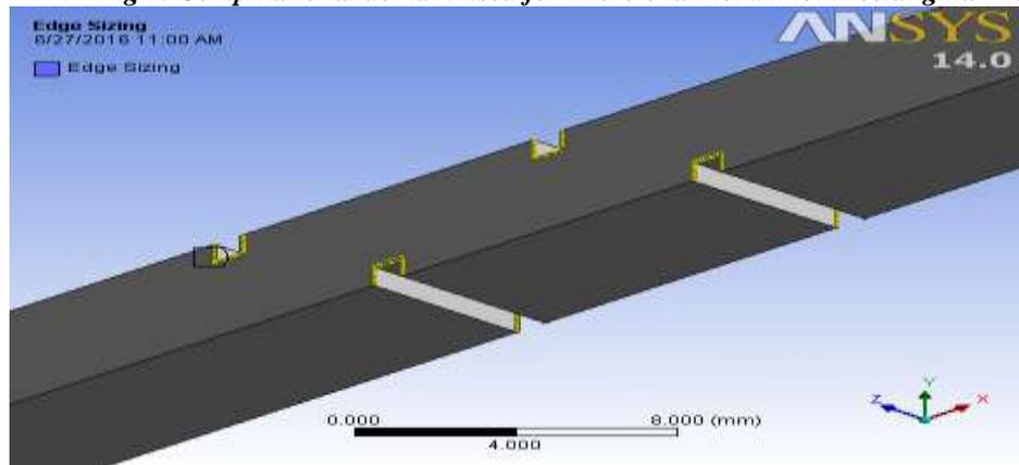
**Fig 2: Computational domain used for the 3D analysis of heat transfer with rectangular ribs**
