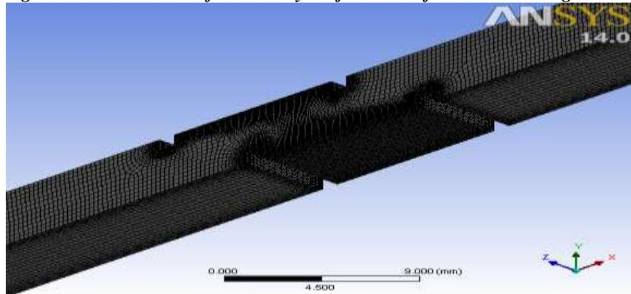
Fig 4: Unstructured mesh for 3d analysis of heat transfer with rectangular ribs
