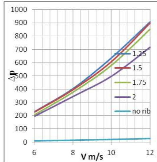
Fig 5.12(b):  $\Delta p$  v/s V plots for rib length 0.4 & 0.5
