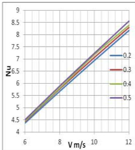
Fig 5.2 (a): Nu v/s V plot for rib pitch=1.25
