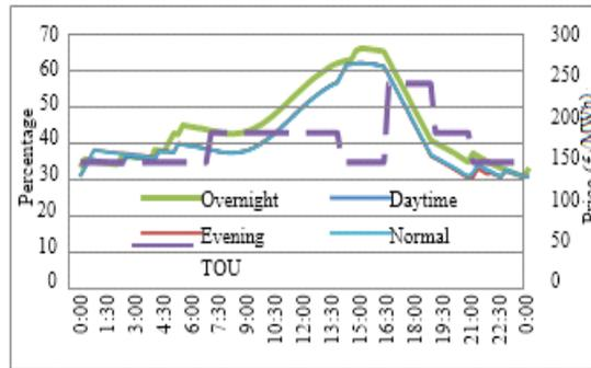
Fig.15 SOC of battery in EMS system with 89% efficiencies
