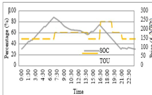
Fig. 8. SOC of battery in normal house.
