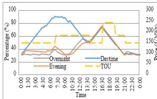
Fig. 17. SOC of electric heating house with large PV output
