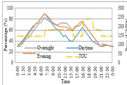
Fig. 10. SOCs of battery in houses with heat load.
