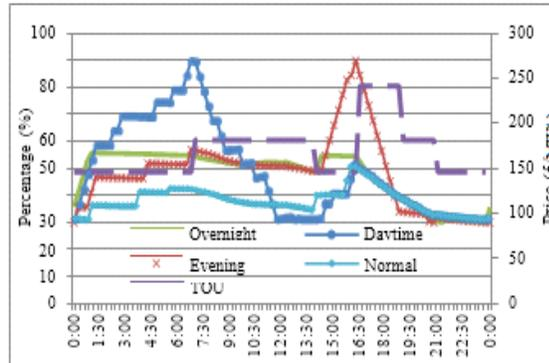
Fig.14. SOC of larger battery
