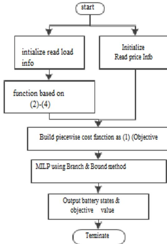
Fig. 5. Flowchart of optimization method
