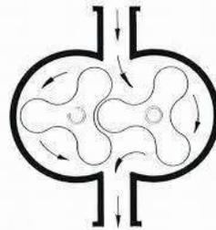
Passage of Air Through a Roots Supercharger
