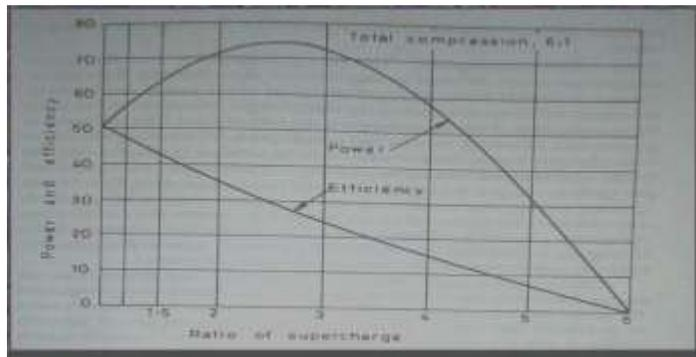
Figure 14. Effect of supercharging ratio on power and efficiency
