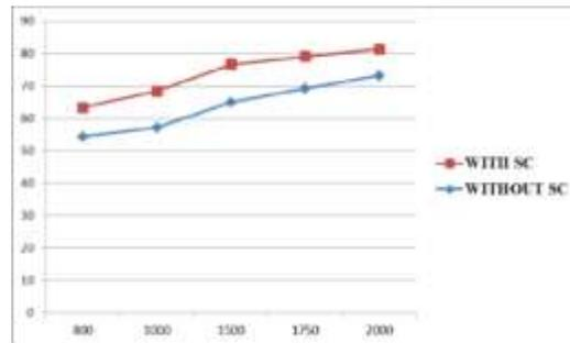
Fig. 6 mechanical efficiency vs rpm
