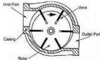
*Fig. 3 Vane Supercharger*
