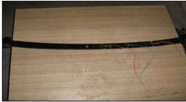
**Figure: 6.2 Leaf spring with strain gauges mounted.**
