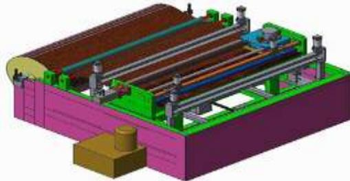
**Figure 2. CAD (CREO) Model Showing Conceptual Design of Leather cutting machine.**
