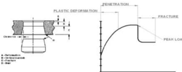
Figure 6. Load curve of cutting force of blanking or piercing punch
