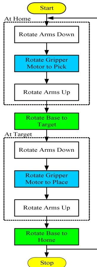
Figure 3. Flowchart of the robot operation.
