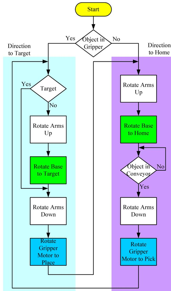
Figure 6. Flowchart of the robot operation.
