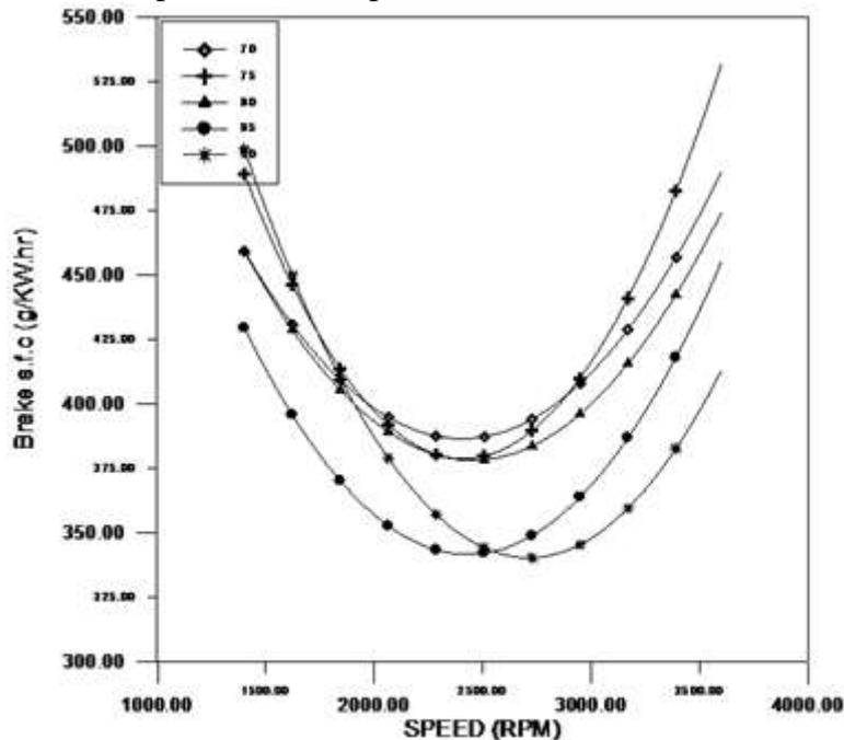
Fig.(7): Relationship between speed and Brake specific fuel consumption
