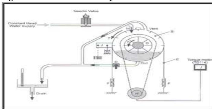
**Fig.(1): Testing the hydraulic performance transaction device type (TD115)**
