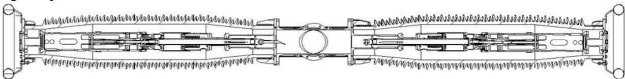
Figure 1 Section of high voltage gas interrupter
