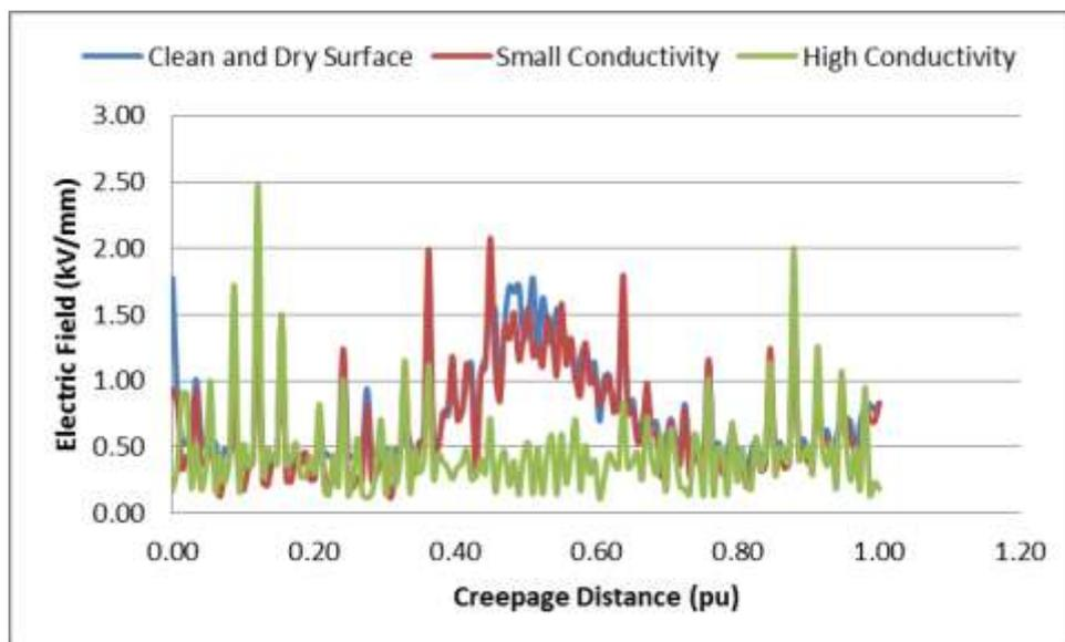
Figure 4 Electric Field curve for different environments
