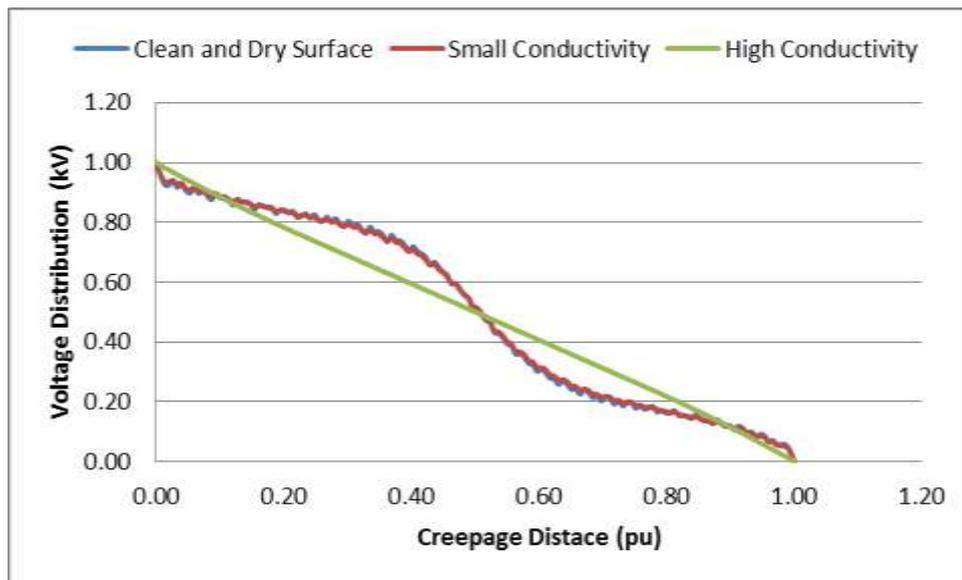
Figure 4 Voltage curve for different environments
