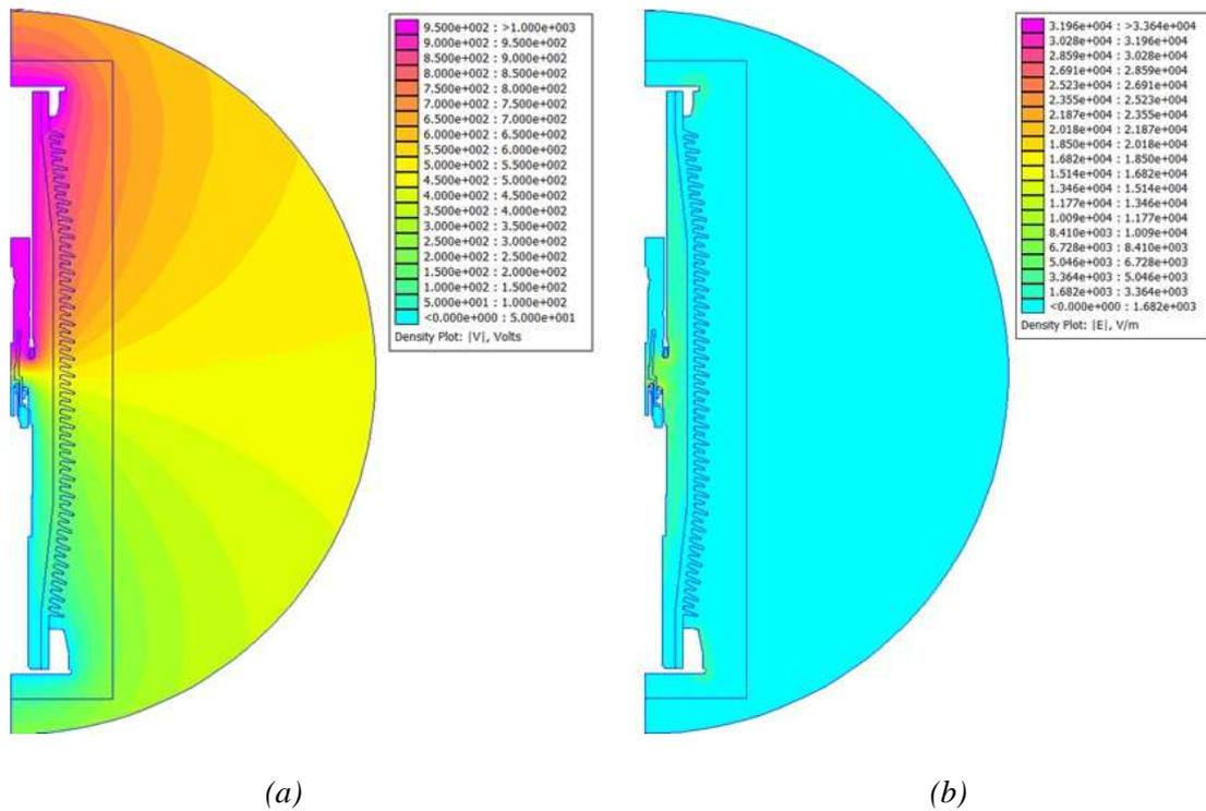
Figure 3 (a) Voltage density plot (b) Electric field density plot
