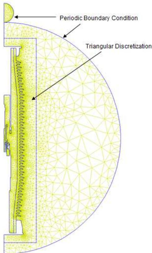
Figure 2 Axisymmetric model of high voltage insulator
