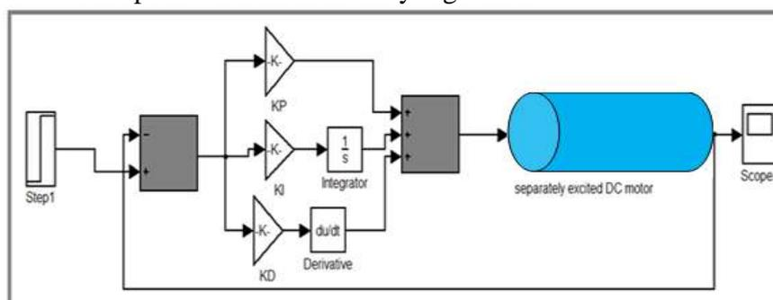
Fig 1 PID controller with DC motor
