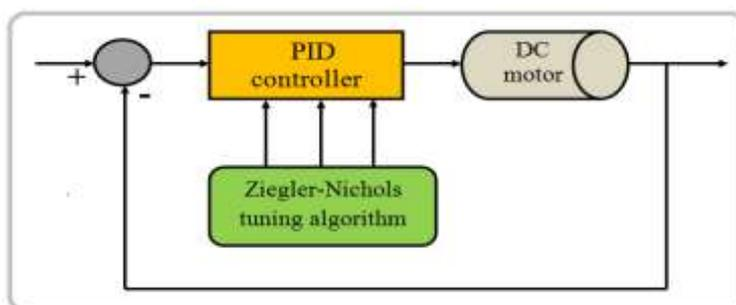
FIG 3.Zeigler Nichols algorithm with PID controller [9]
