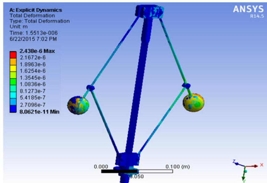
Fig IV.I: Total deformation
