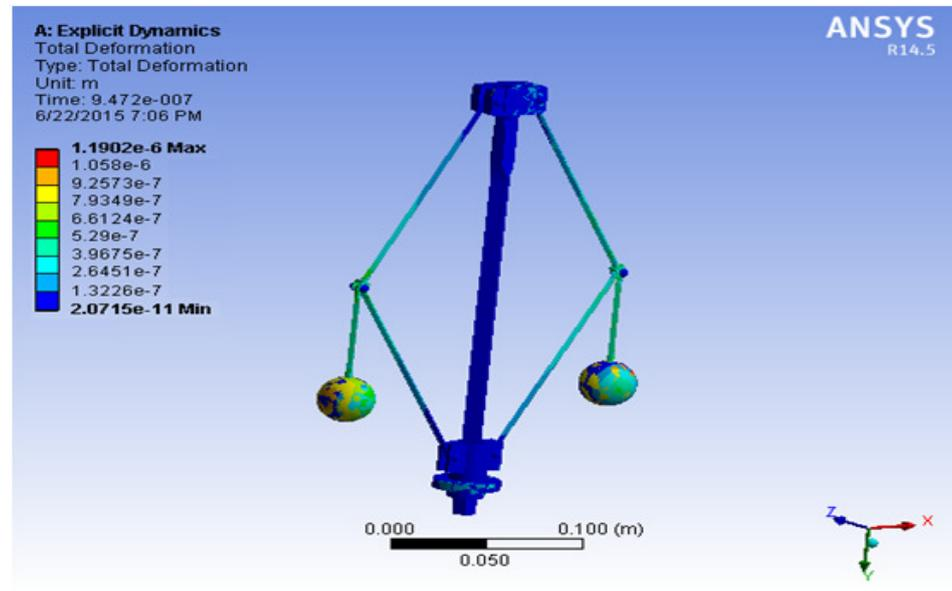
Fig V.I: Total deformation
