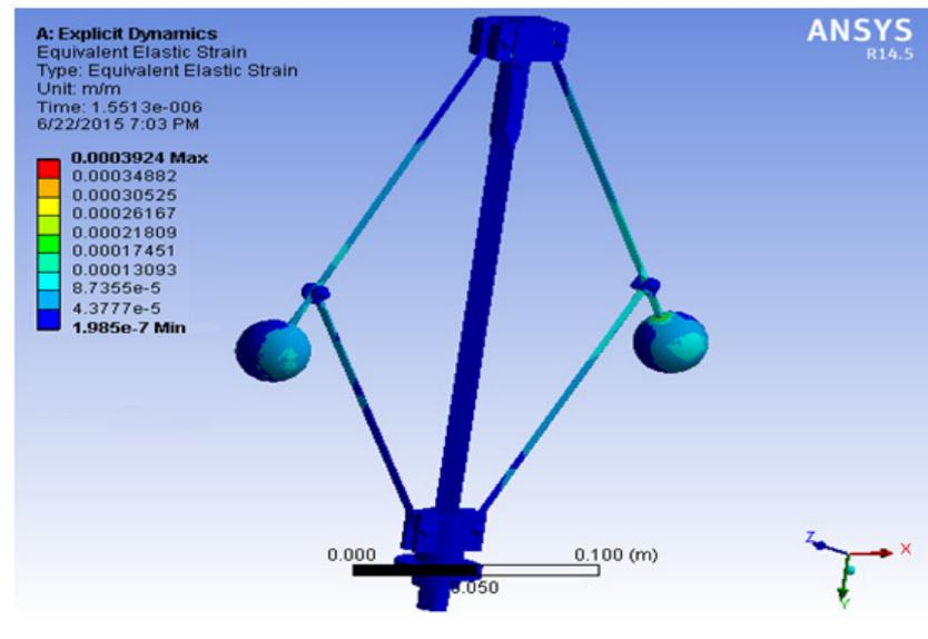
Fig IV.II equivalent elastic strain
