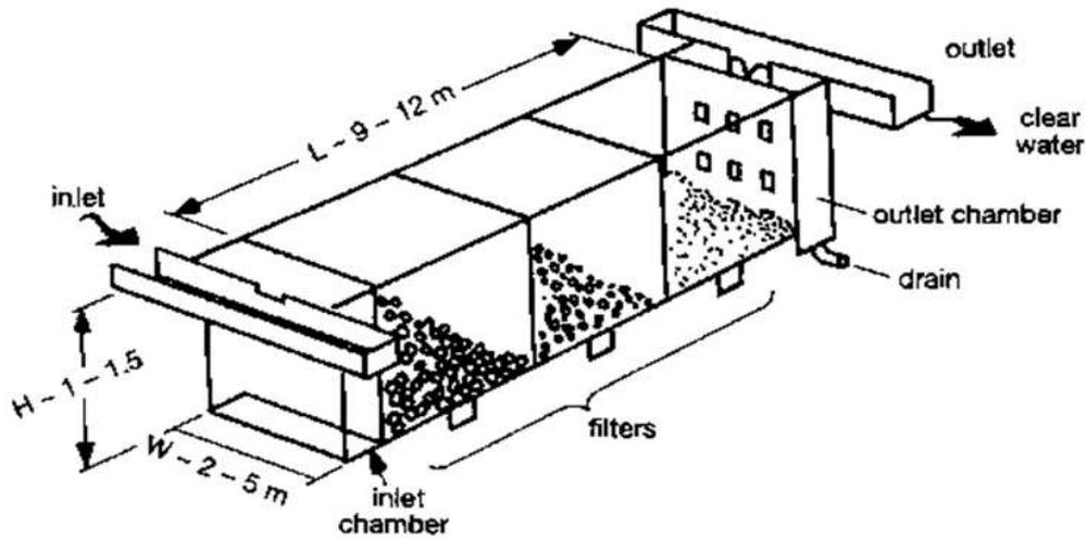
Fig 1: Horizontal roughing filter (Source: Internet)
