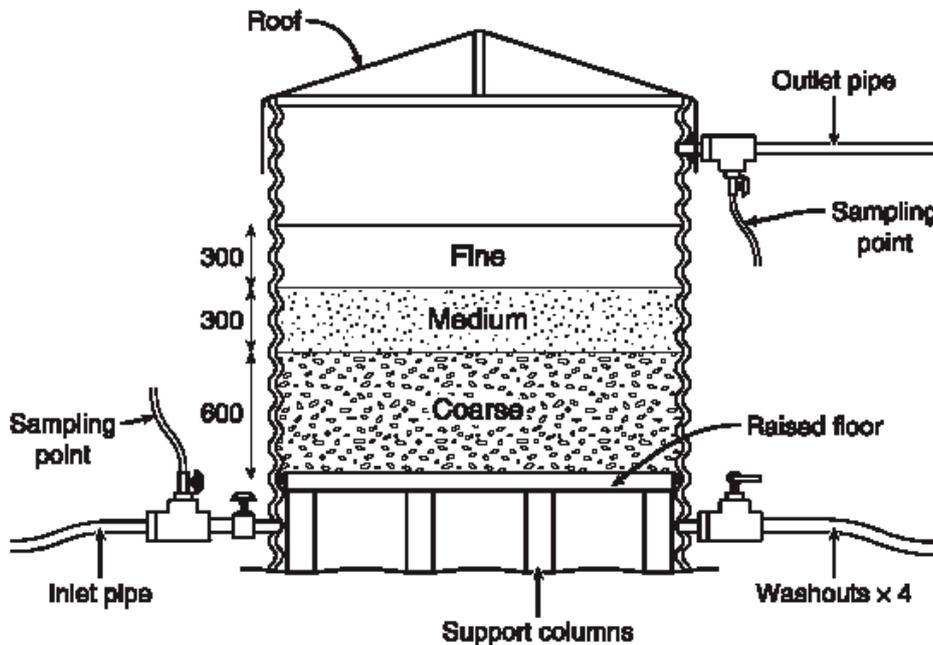
Fig 2: Vertical roughing filter (Source: Internet)
