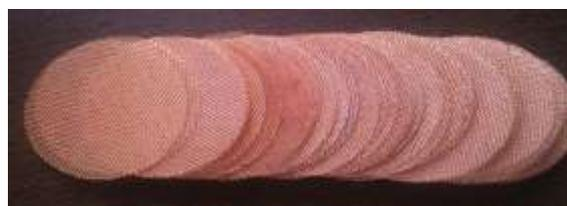
From this research it was concluded that the use of copper based catalytic converter reduces emissions of HC by 38% and CO by 33%.
