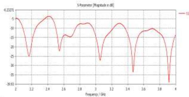
Figure 3 S Parameter Value of Square Shaped Microstrip Patch Antenna
