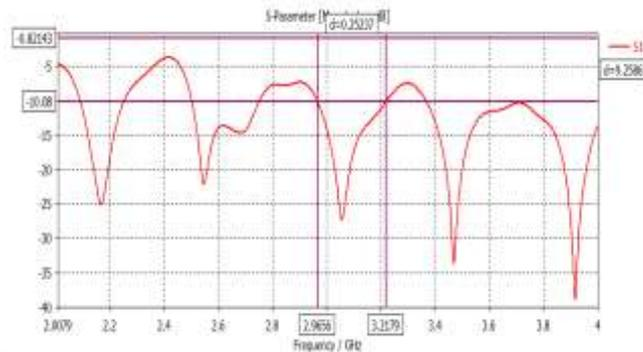
Figure 4 Bandwidth of Square Shaped Microstrip Patch Antenna
