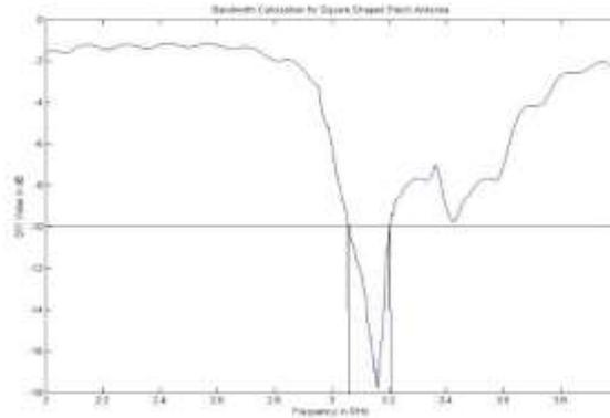
**Figure 6 Bandwidth of Square Shaped Microstrip Patch Antenna**
