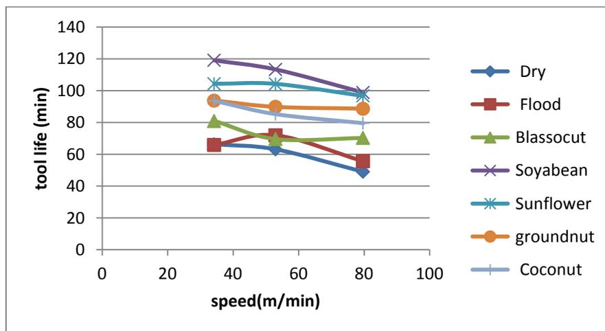
Figure 3. Variation of tool life at different cutting speed
