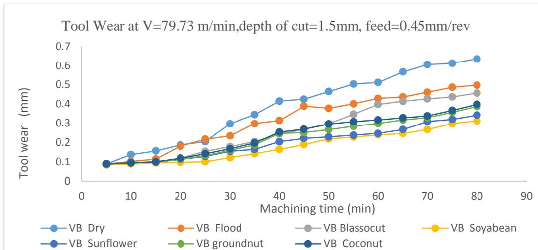
Figure 2 Variation in tool wear ( $V=0.79.73\text{m/min}$ ,  $f=0.45\text{ mm/rev}$ ,  $dp=1.5\text{ mm}$ ).
