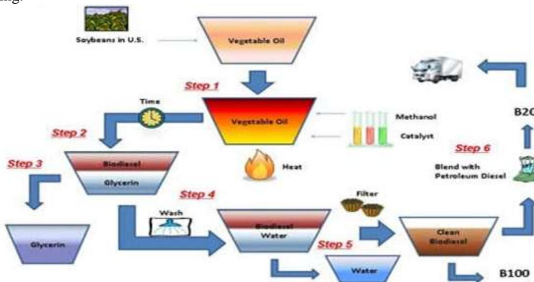
Fig 2. Biodiesel production process
