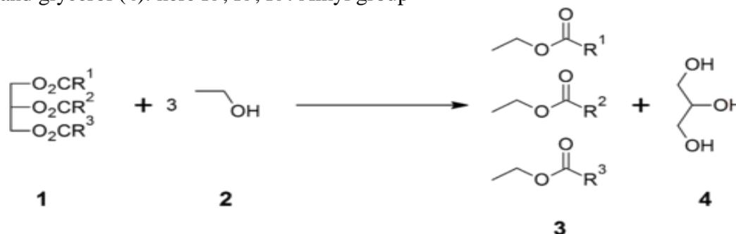
The alcohol reacts with the fatty acids to form the mono-alkyl ester (biodiesel) and crude glycerol. The reaction between the bio lipid (fat or oil) and the alcohol is a reversible reaction so excess alcohol must be added to ensure complete conversion.
