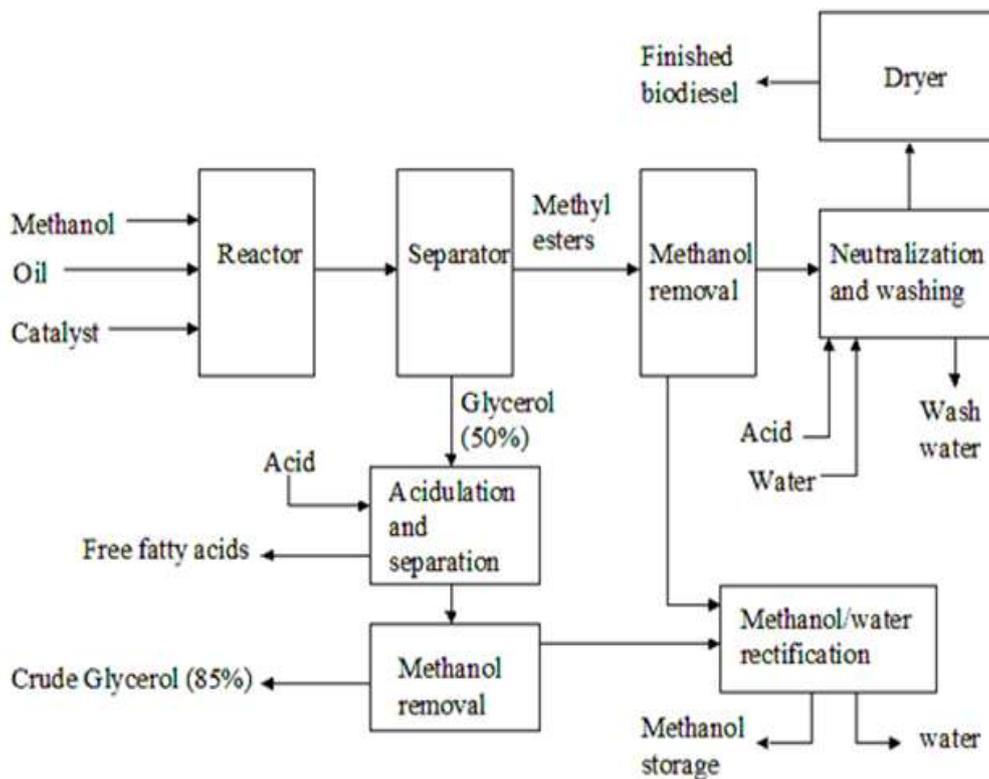
Fig.5 Biodiesel production by highly acidic oils or fats
