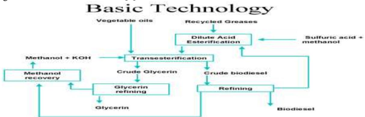
FIG.3 Biodiesel production by free fatty acids
