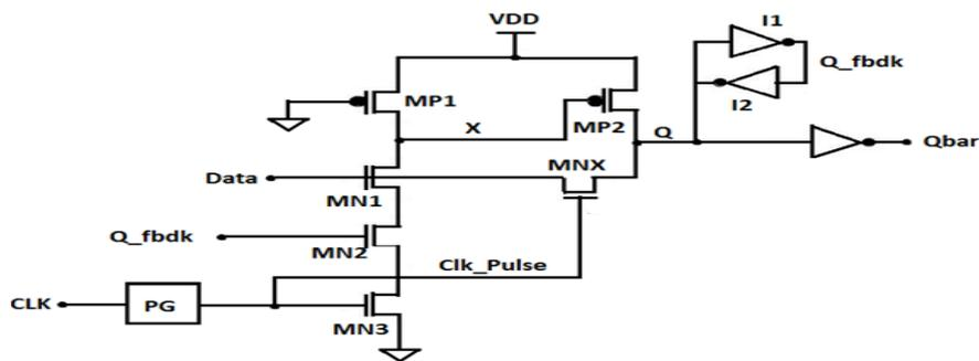
**Fig.1.** Pulse triggered flip-flop(P-FF)
